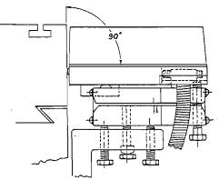
Use the Tilt Screw, if necessary, to orient properly. (Be sure to loosen the Clamp Screw first if raising the Tilt Screw.)
