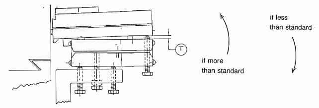
4. Pry the Trav-A-Dial away from the Running Surface and while the wheel is not touching, move it a small amount to change the Gage Wheel Track.
