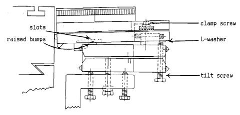
The Tray-A-Dial should fit with the raised bumps of the M-5 Base in the slots on the underside of the Trav-A-Dial, the Clamp Screw screwed into the hole of the M-5 Base, and the Tilt Screw of the M-5 Base in contact with the hardened L-Washer.
