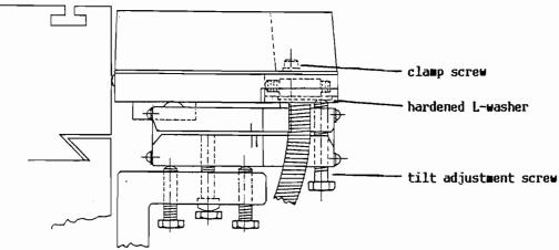
The Clamp Screw is screwed into the M-5 Base, and the Hardened L-Washer is in contact with the Tilt Adjustment Screw.
