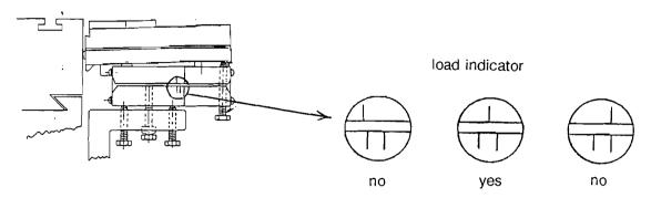
4. Tighten the clamp screw until the load cell washers become flat.
