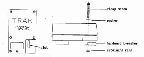
2. Place the TRAK Sensor on the M-5 Base. The TRAK Sensor has one slot on the underside and one flat that fit over the raised bumps of the M-5 Base. Screw in clamp screw to be snug, but not tight. Push the TRAK Sensor so that the Gage Wheel is in contact with the Running Surface.
