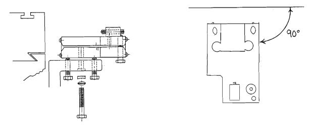
3. Use a bubble level to align the raised bumps on the M-5 base with the Machine Tool surface.
