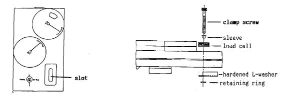
2. Place the Trav-A-Dial (with clamp screw assembly) onto the M-5 Base. Screw in clamp screw to be snug, but not tight. Push the Trav-A-Dial so that the Gage Wheel is in contact with the Running Surface.
