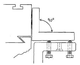
2. Place the M-5 Base on the pusher screws and screw in the puller screws.
