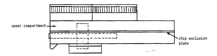
The Chip Exclusion plate is sealed by a rubber gasket which fits along the case.
