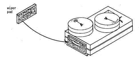
After installation this wiper pad is filled with oil. It forms a lubrication system which wipes the running surface clean as it passes.
