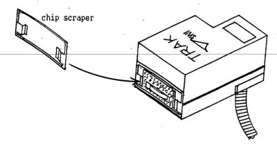
The TRAK Sensor also employs a metallic Chip Scraper which pushes metal chips away and breaks long, stringy chips.
