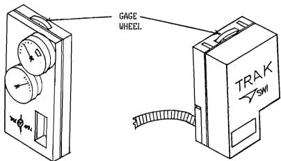
The gage wheel is made from tool steel. It is hardened to 63C on the Rockwell Hardness Scale.
