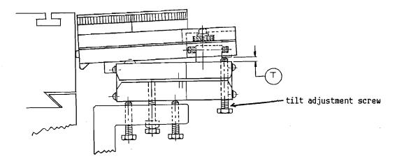
The adjustments are made by the Tilt Adjustment screw on the Mounting Base.
