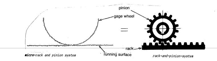
When this pattern is formed, the Gage Wheel is operating in its own "micro-rack-and-pinion" system.
