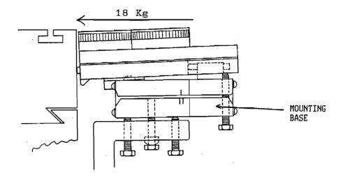
After the Gage Wheel has rolled over its running surface a few times it forms a track or rack in its own image. This is because the hardness of the Gage Wheel and its pushing force actually deform the running surface. This "rack" is small, less than .04mm of depth.
