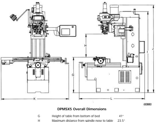
H Maximum distance from spindle nose to table 23.5<sup>°</sup>
