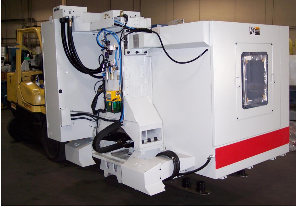
Figure 5 – Lifting the TMC
