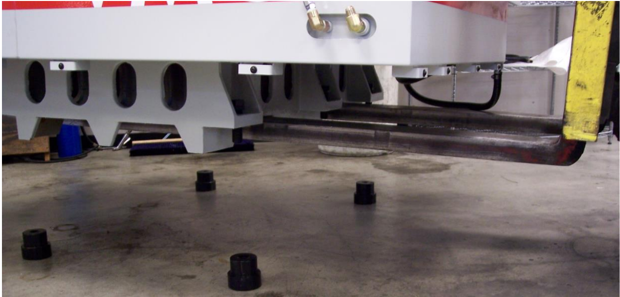
Figure 3 – Lifting the TMC
