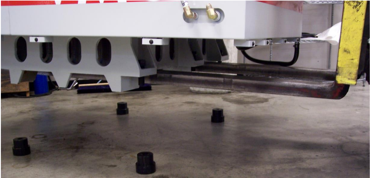
Figure 3 – Lifting the TMC
