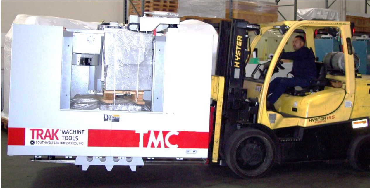
Figure 4 – Lifting the TMC
