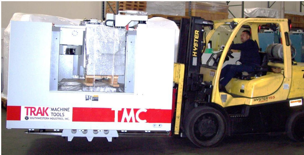
Figure 4 – Lifting the TMC
