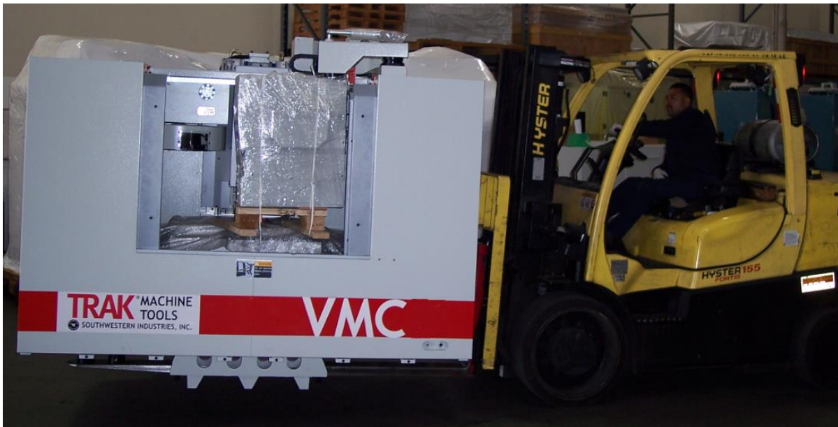
Figure 4 – Lifting the VMC
