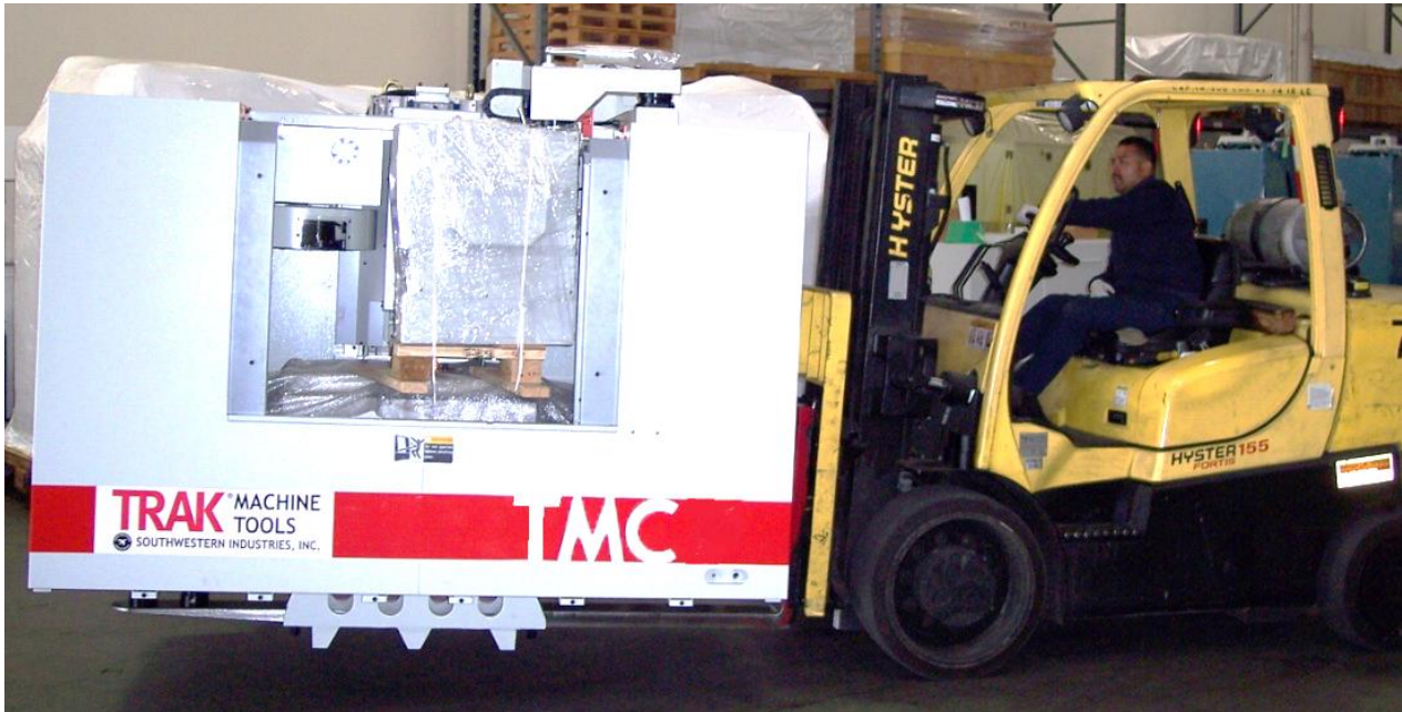
Figure 4 – Lifting the TMC
