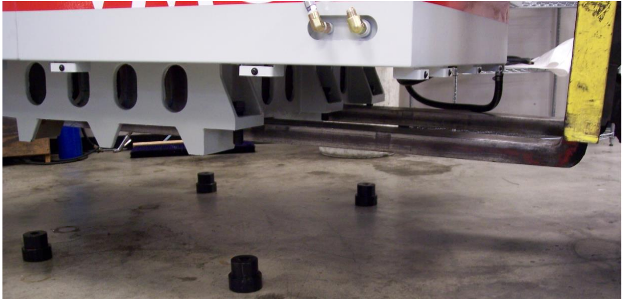
Figure 3 – Lifting the TMC
