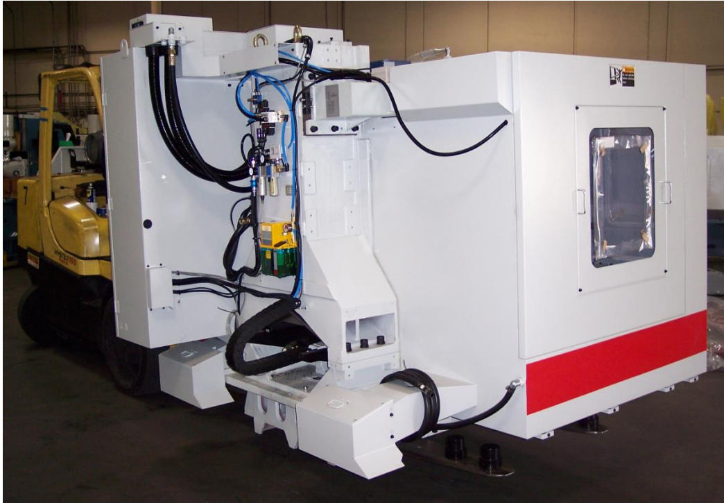
Figure 5 – Lifting the TMC
