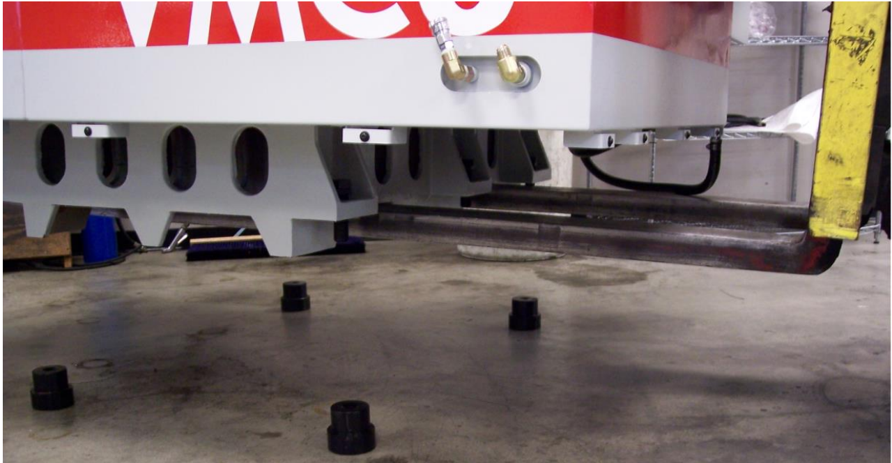
Figure 3 – Lifting the VMC
