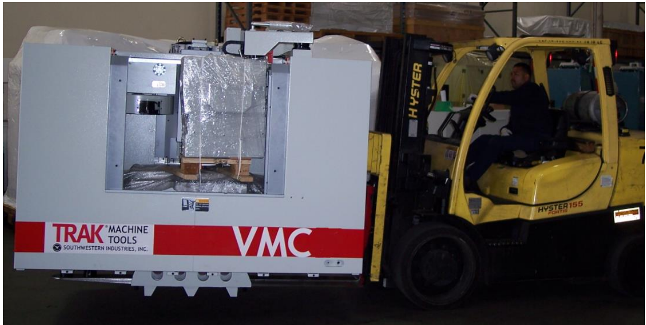
Figure 4 – Lifting the VMC
