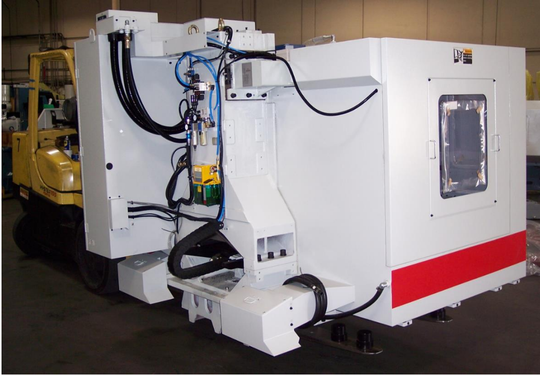
Figure 5 – Lifting the TMC
