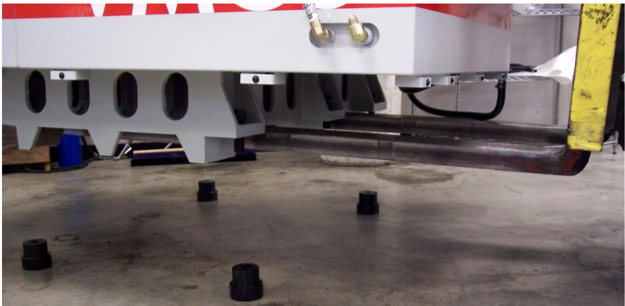
Figure 3 – Lifting the TMC
