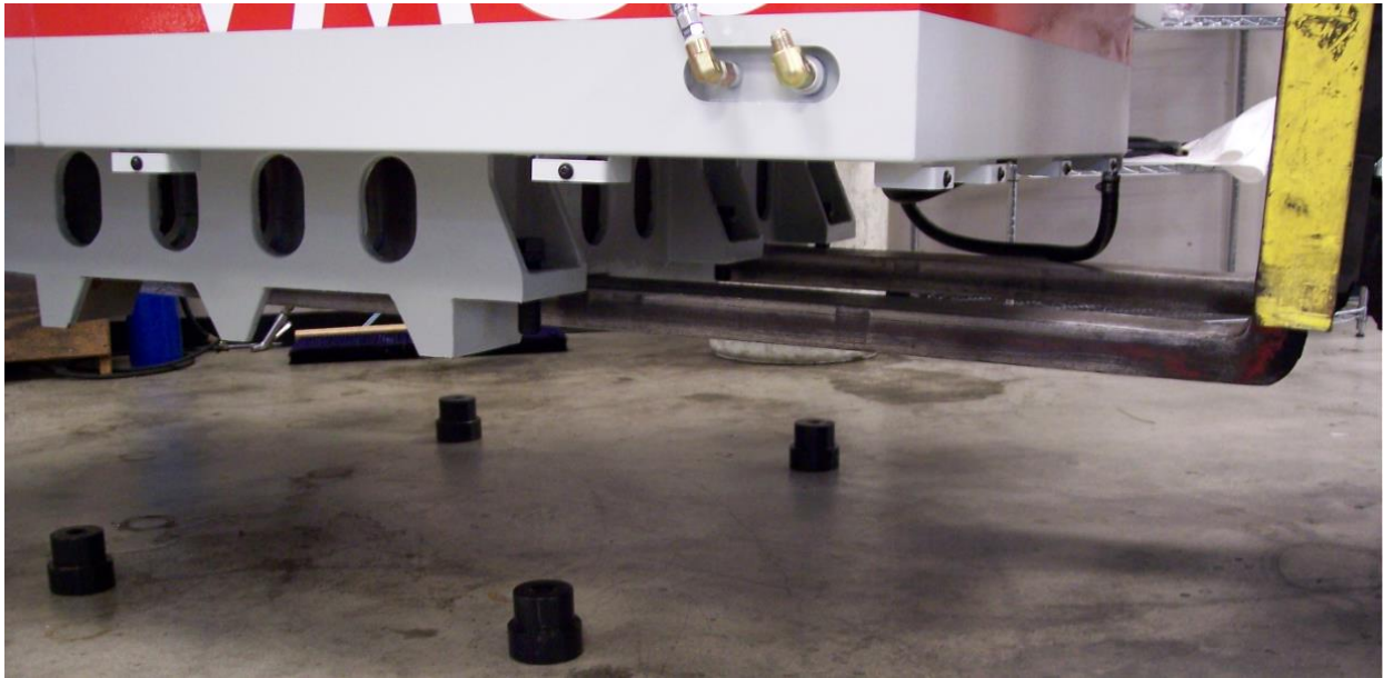
Figure 3 – Lifting the TMC
