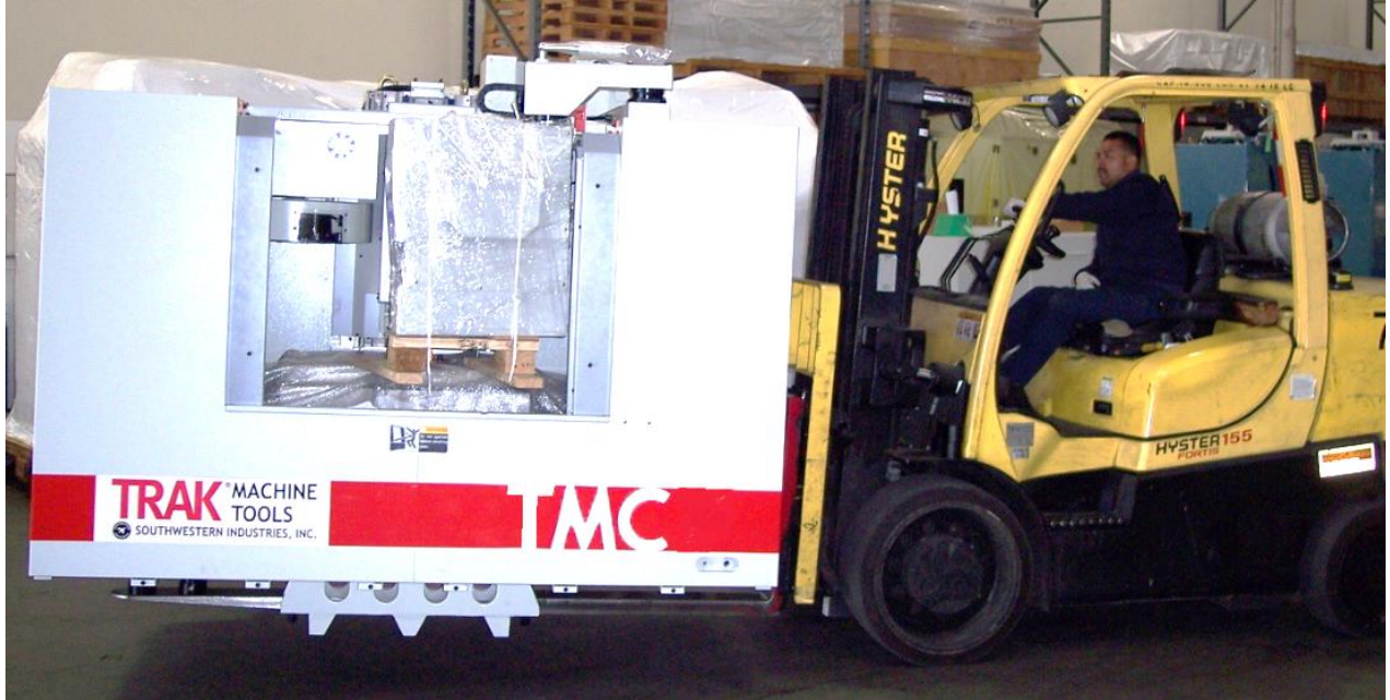
Figure 4 – Lifting the TMC
