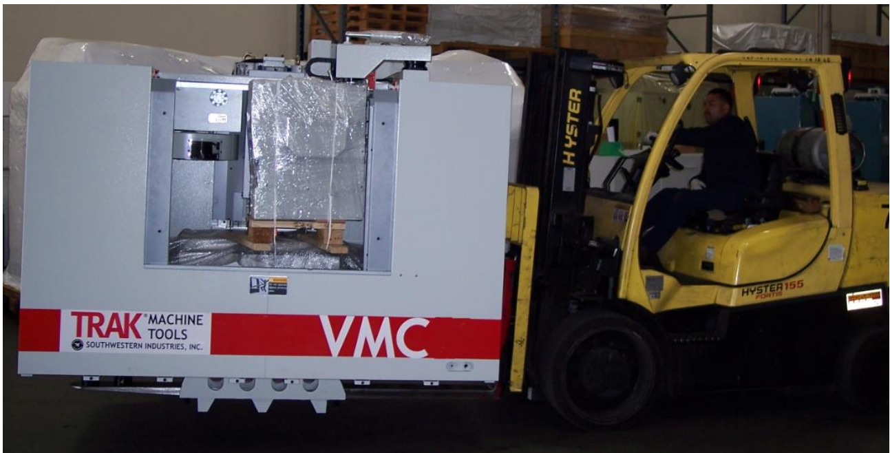
Figure 4 – Lifting the VMC
