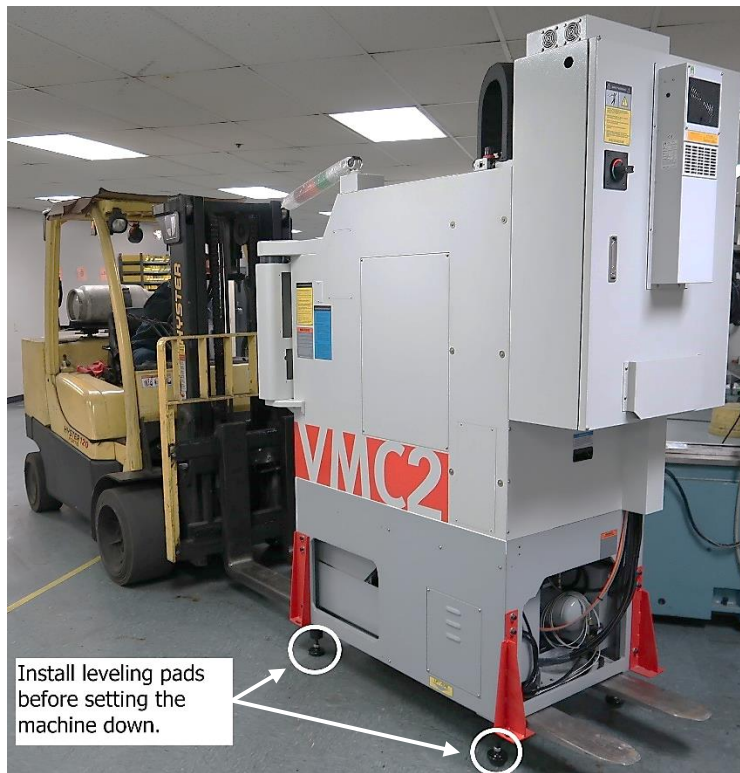
Figure 3 – Installing Leveling Pads
