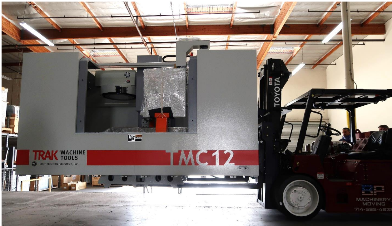
Figure 4 – Lifting the TMC
