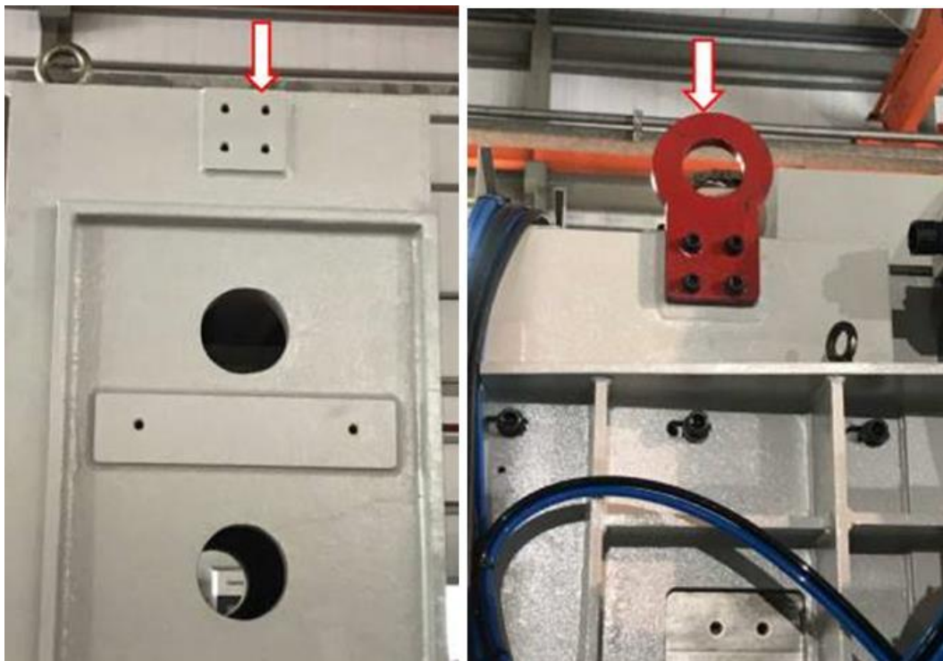
Figure 8 – Lifting Machine on Top of Column
