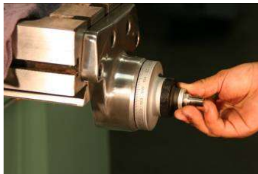
Vernier dial, lock nut, spacers as needed
