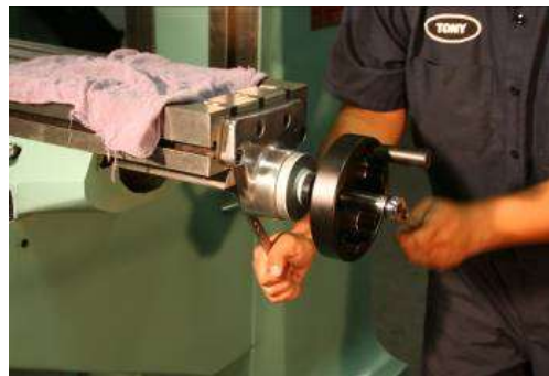
Tighten, don't push down Torque to 20 ft/lbs
