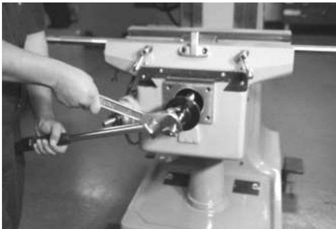
Torque clamp nut to 50 ft/lb.
