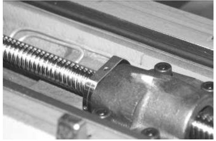
Install set screw flush, not tight
