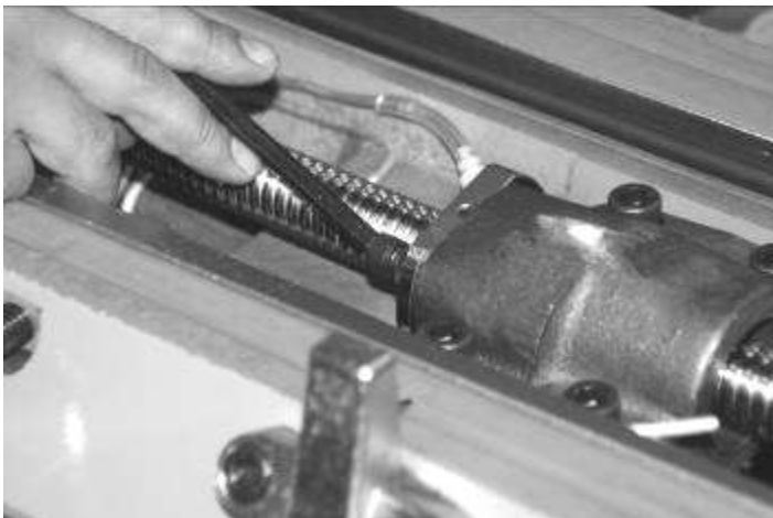
Tighten ball nut retaining screw
