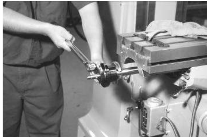
Tighten, don't push down, to 50 ft-lbs
