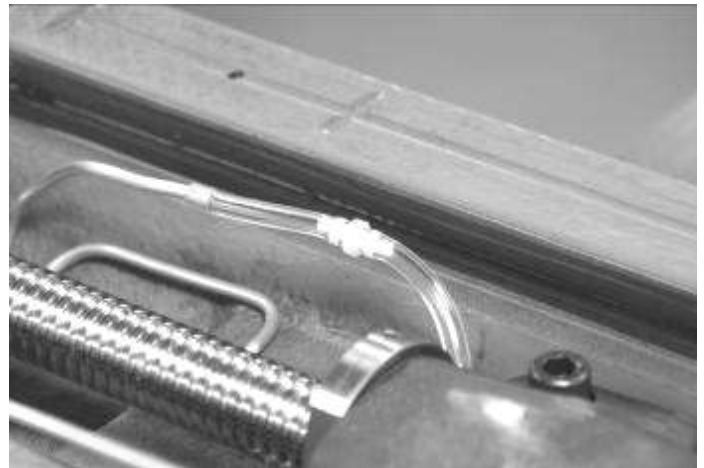
Oil line installed with restrictor
