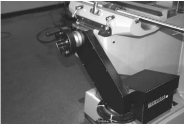
Y-axis drive completed
