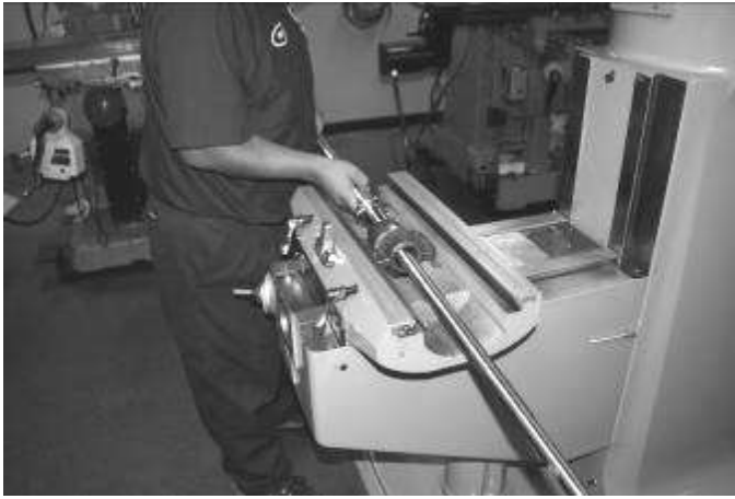
Position ballscrew with yoke still loose
