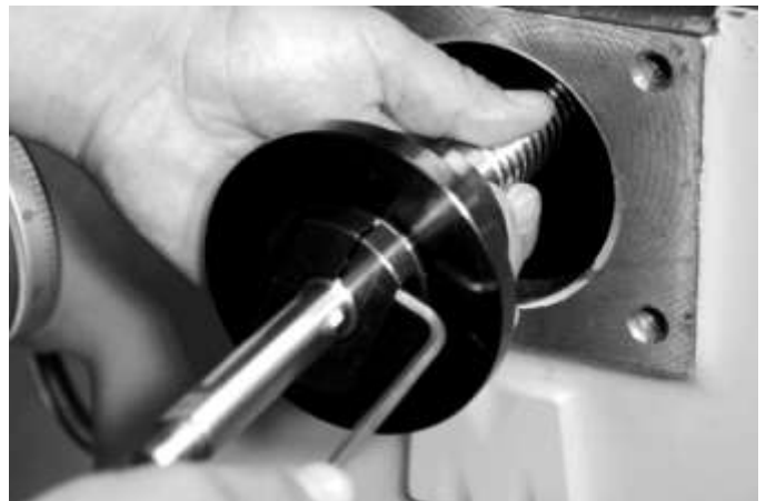
Torque socket head cap screw to 90 in/lb.
