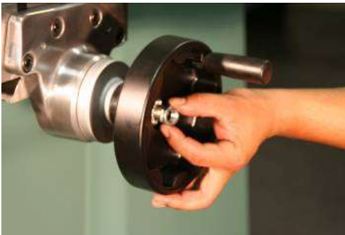
Handwheel, washer, star washer, nut
