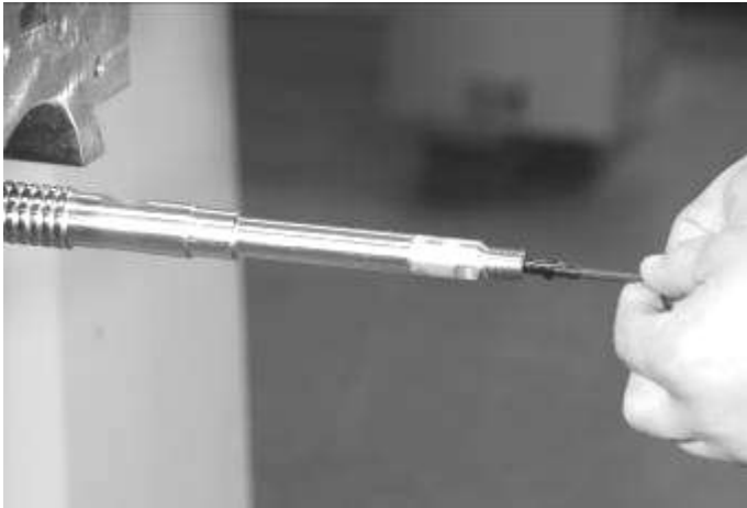
Set screw to tighten extension
