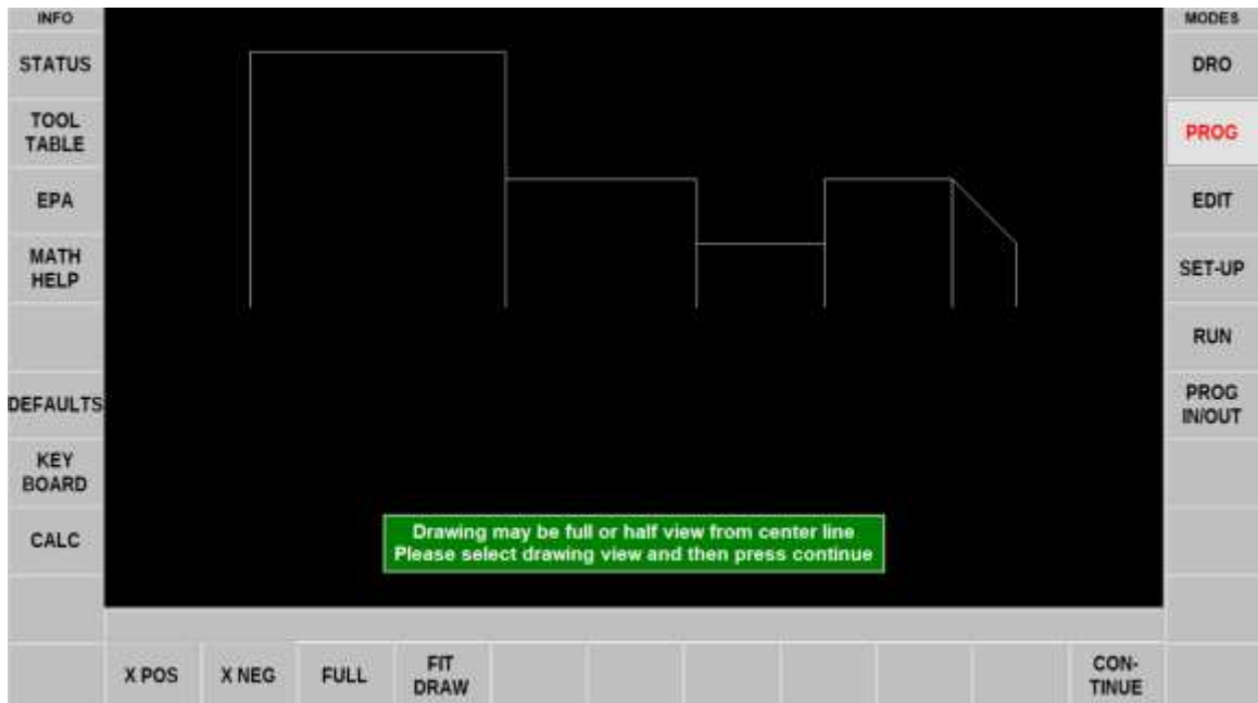
FIGURE 4.6.2 The X neg key will display the portion of the drawing from the ABS 0 point you specified, up.
