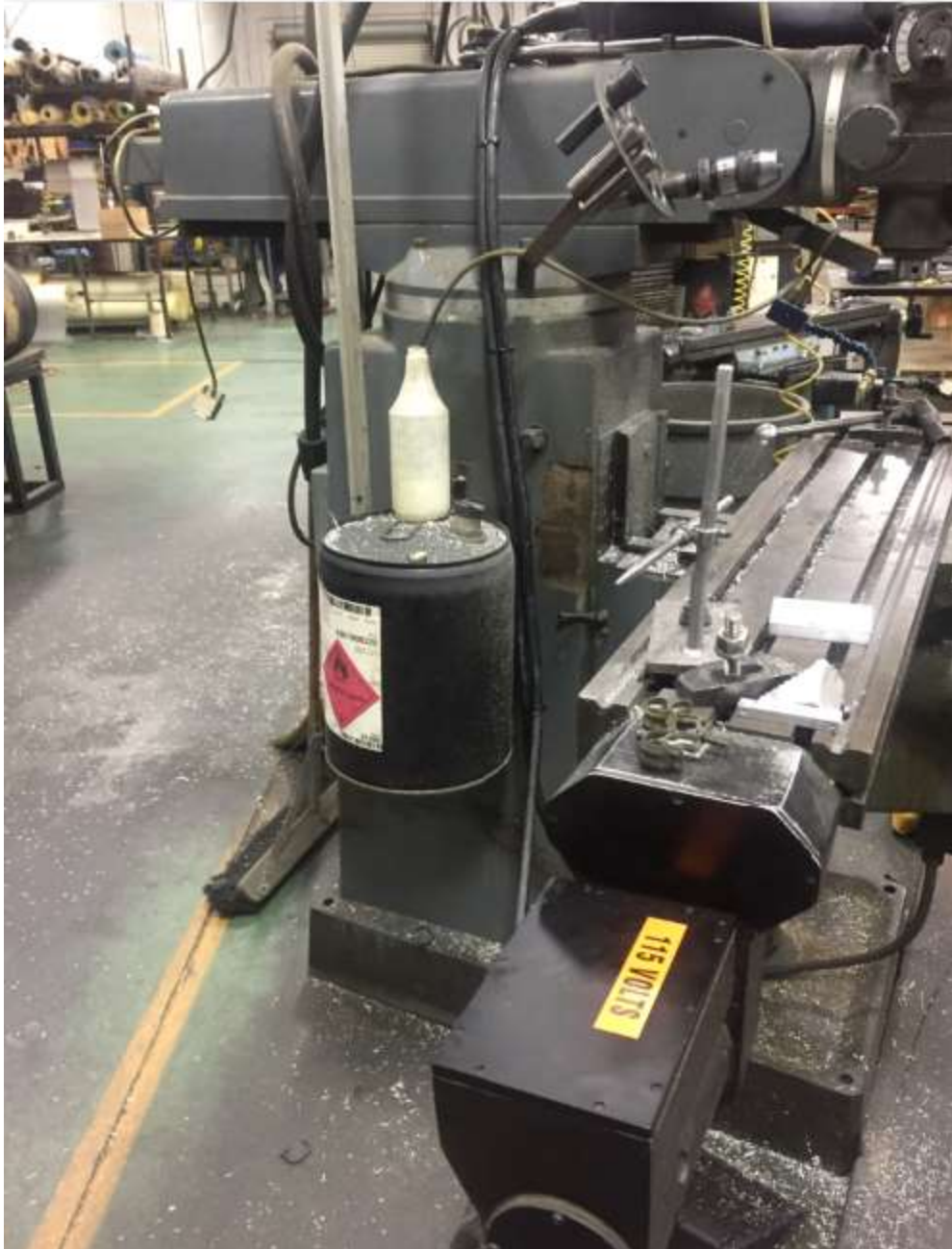
Routing of X and Y Axis Motor Cables on Knee Mill
