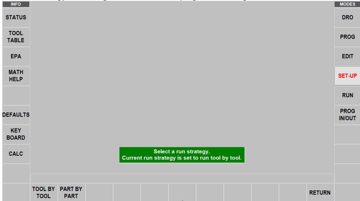
Figure 12.5 - ProtoTRAK RMX displaying run strategy soft keys with Tool by Tool run strategy set.
