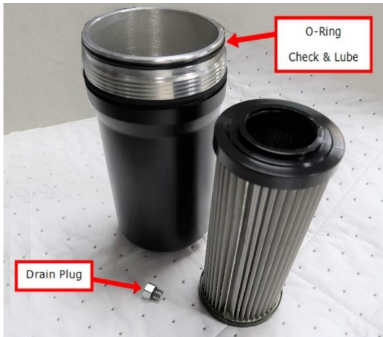
Figure 7.3 – Filter Canister and Element
