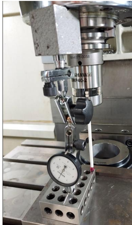
Figure 9.2.2 – Calibration check using dial indicator on spindle base
