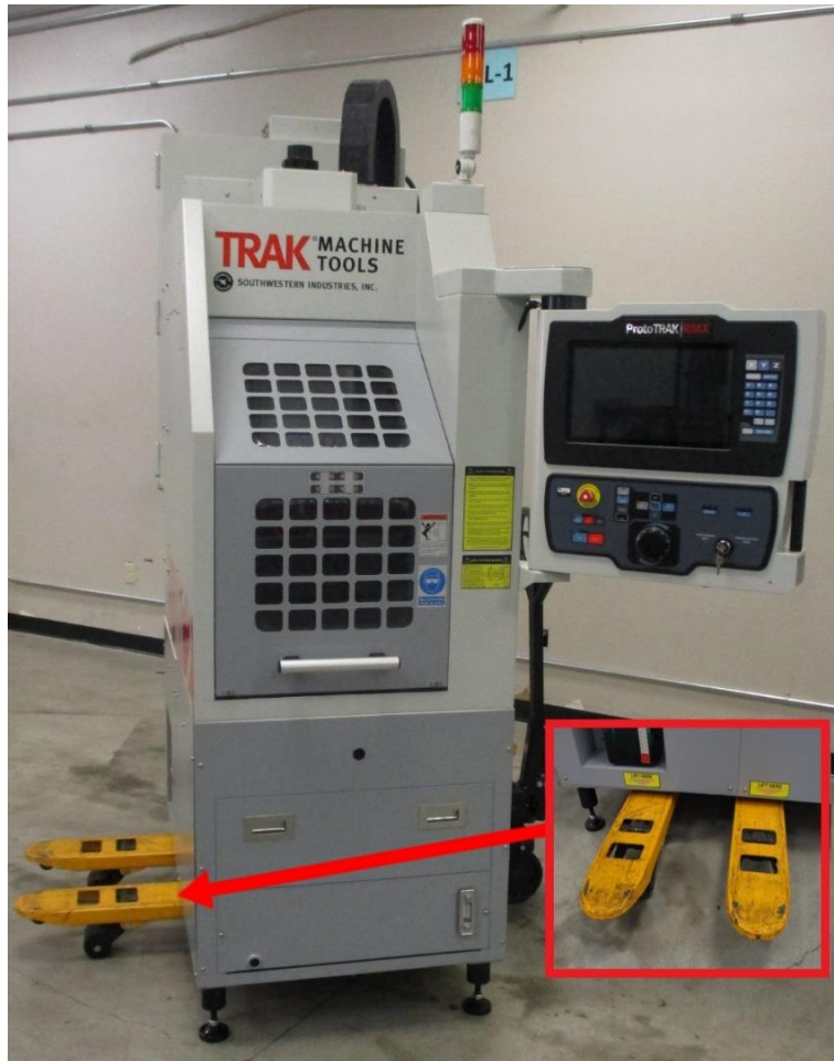
Figure 2.4a - Detail of Lift Blades Set Under VMC2 with Proper Lift Points
