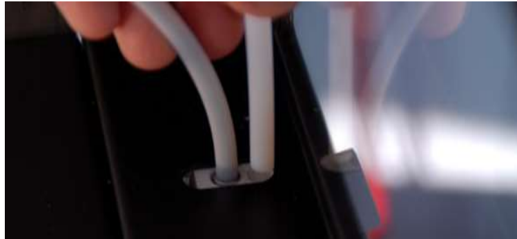
Figure 3.8 Fitting PTFE piping into motor assembly as shown
