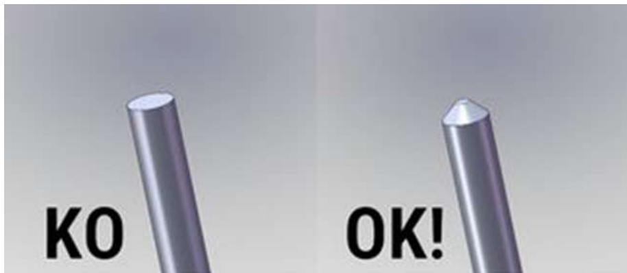
Figure 2.3.3 Illustration of correct and incorrect filament tip sharpening
