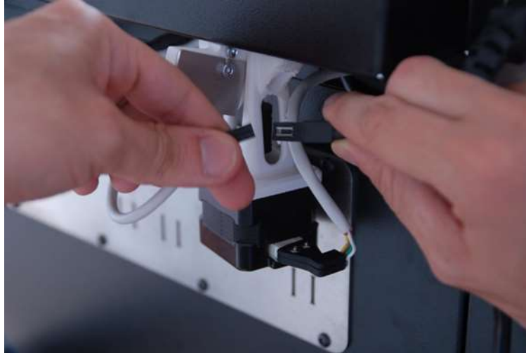
Figure 3.7 Connect Stepper Motor and Filament Sensor
