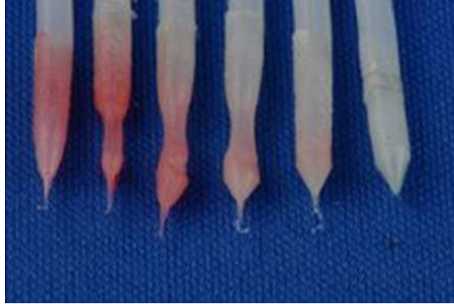
Figure 2.4.7 Cleaning Filament Tip Color after multiple Cleaning Cycles
