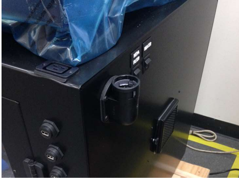
Figure 8.3.3 Printer power outlet on MMS Unit
