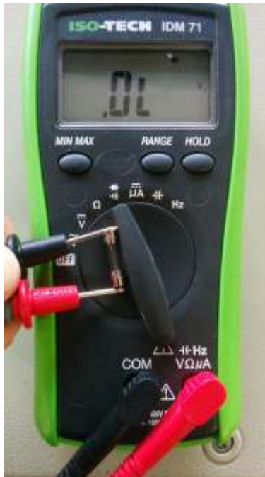
Figure 4.43.3 Multimeter Indicating Blown Fuse
