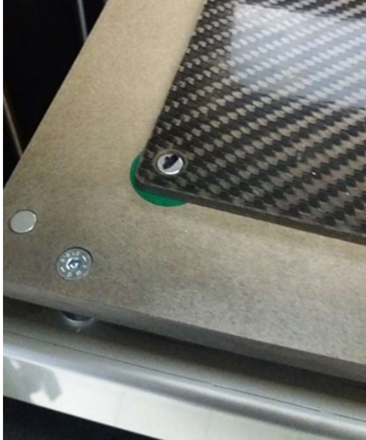
Figure 4.30.6 Plate with Magnet in Corner Hole on Heated Bed
