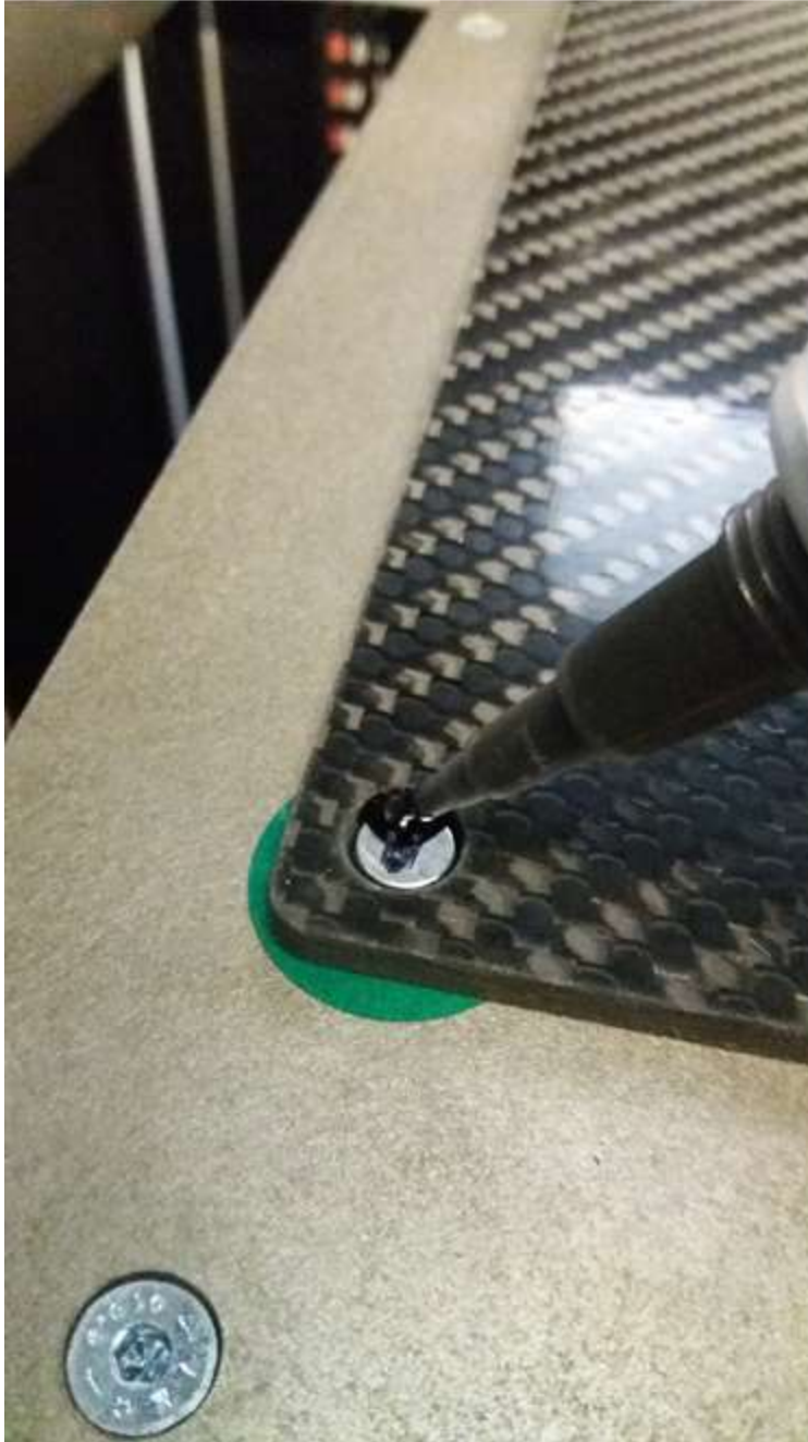
Figure 4.30.7 Applying Glue to Magnet
