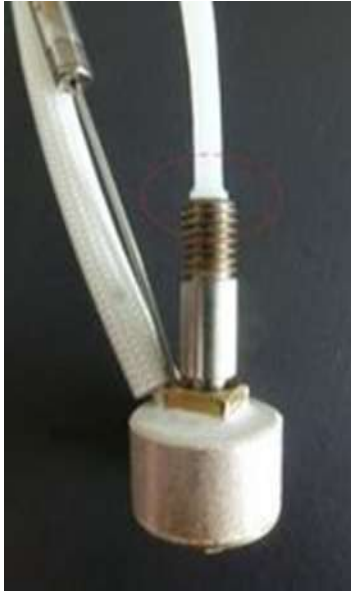
Figure 4.38.1 Extruder with Jam on Entry
