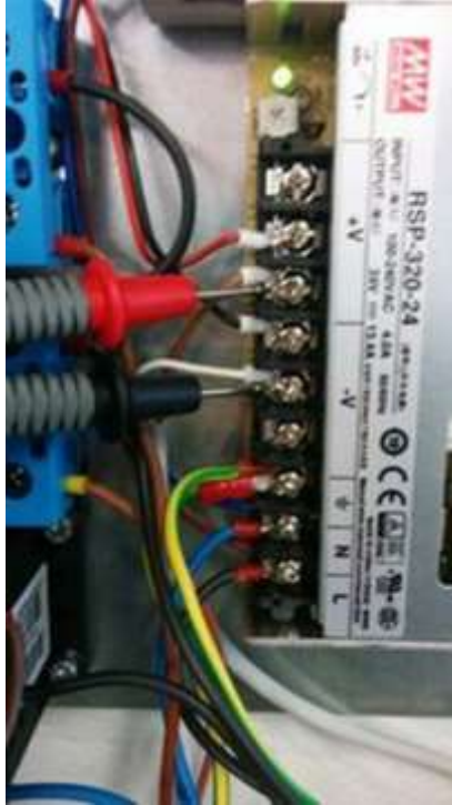
Figure 4.2.13 Check Output Voltage on PSU
