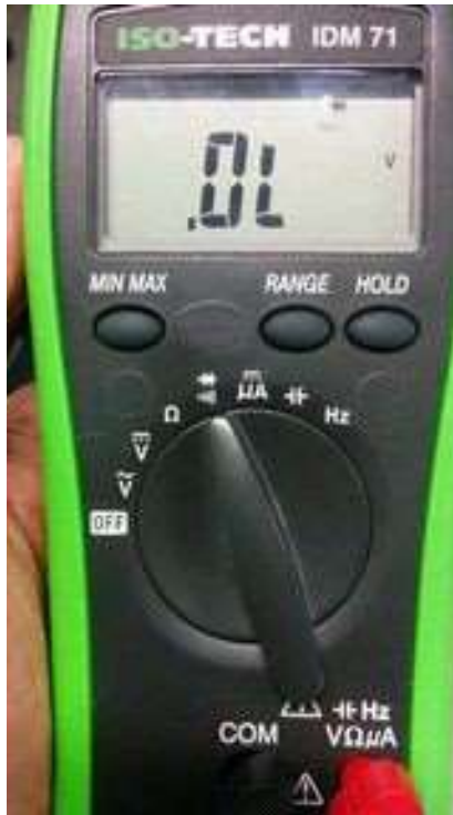
Figure 4.43.1 Multimeter Set to Continuity Mode
