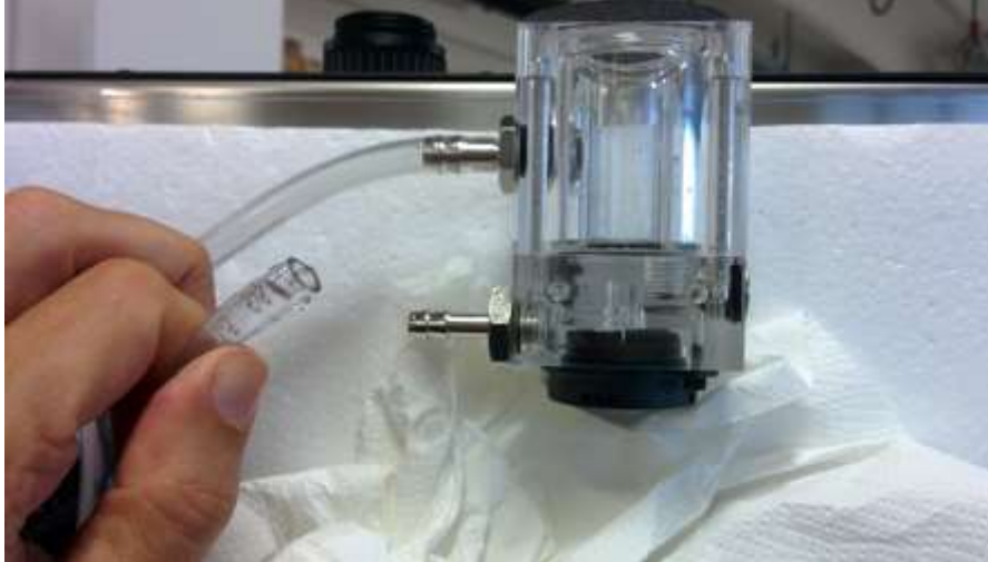
Figure 4.6.10 Detach Outlet Pipe
