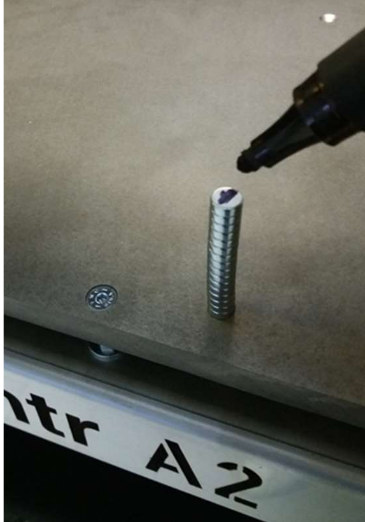
Figure 4.30.4 Mark the Magnet Stack
