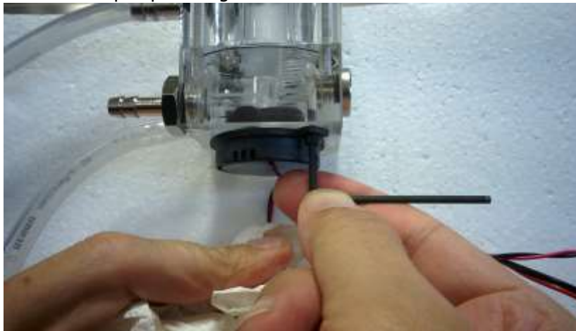
Figure 4.9.5 Removing Pump/Reservoir Screws
