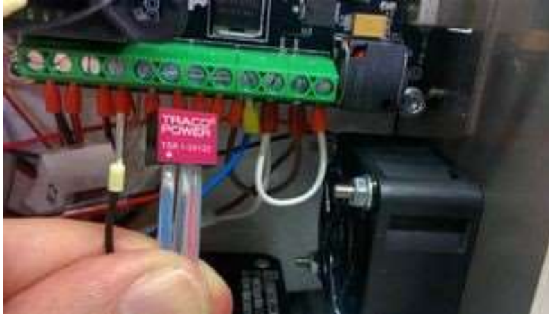
Figure 4.31.6 Auxiliary Power Supply
