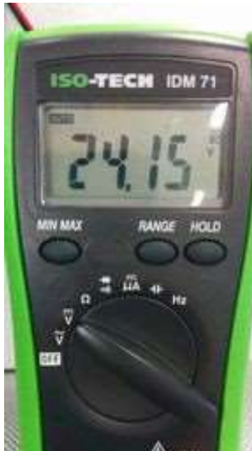
Figure 4.44.4 Correct PSU DC Voltage Indicated on Multimeter
