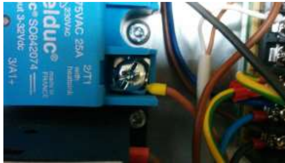
Figure 4.15.5 Correct SSR Cabling Connection
