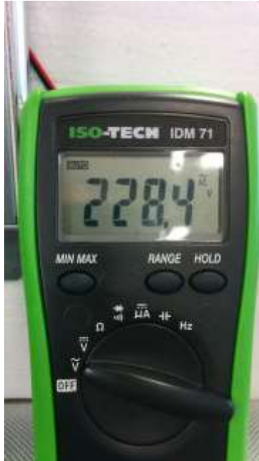
Figure 4.44.2 Correct 228 VAC Entry – MM Set to AC
