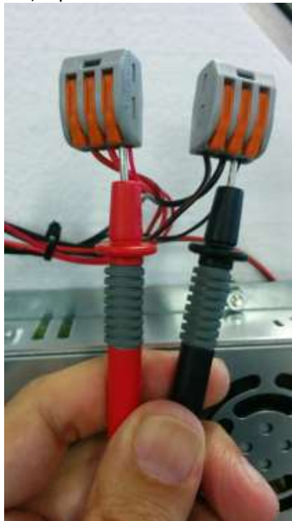
Figure 4.2.14 Check PSU Output Voltage
