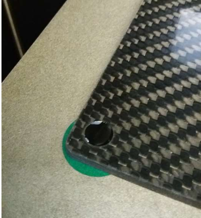
Figure 4.30.8 Completed Glue Application to Plate Magnet
