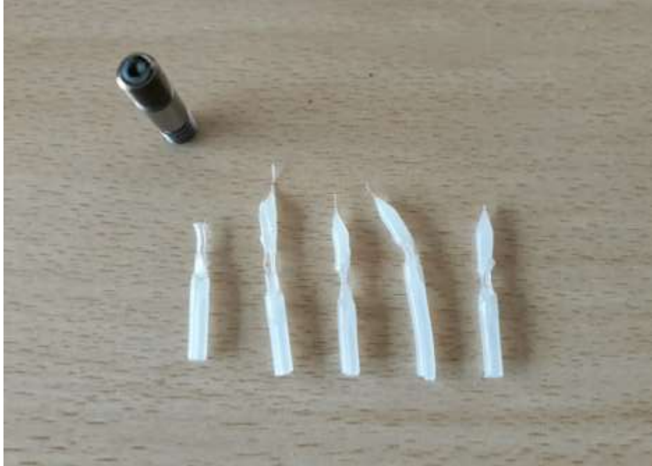
Figure 4.38.3 Poor Cleaning Results Due to Cooling Problems
