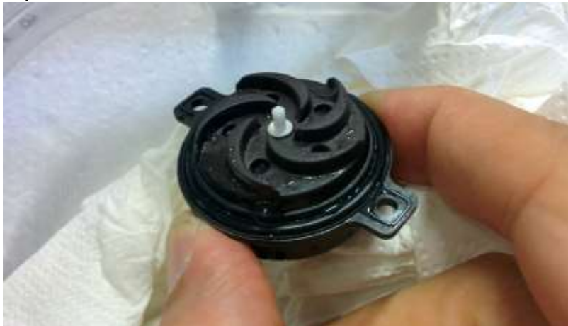
Figure 4.9.7 Clean Pump Sealing Surfaces
