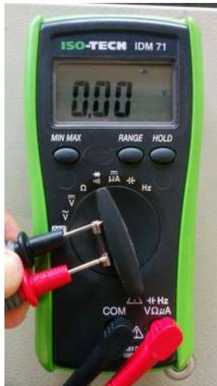
Figure 4.43.4 Multimeter Indicating Fuse OK
