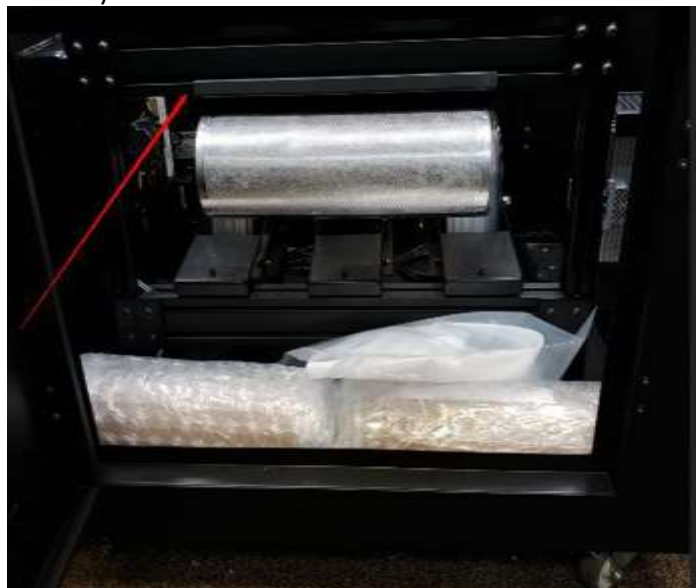
Figure 5.16.25 Desiccant Cylinder Placed in MMS Unit
