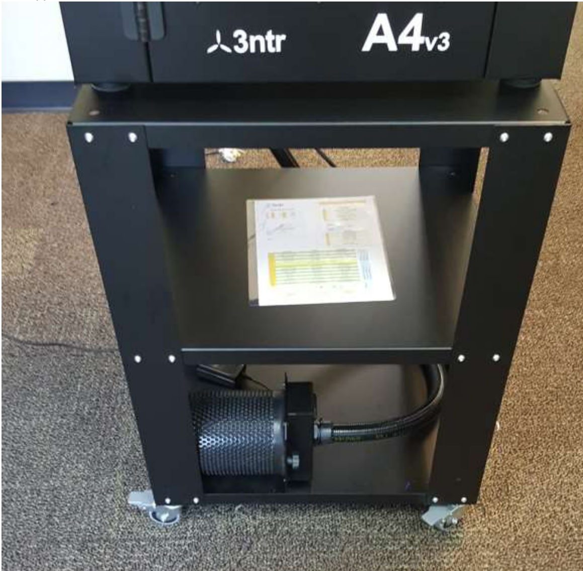
Figure 5.3.10 External HEPA Filter Unit & hose routing on printer stand
