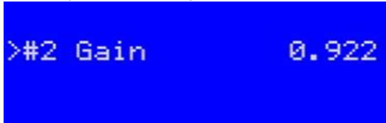
Figure 10.7.3 Modifying Extruder Gain
