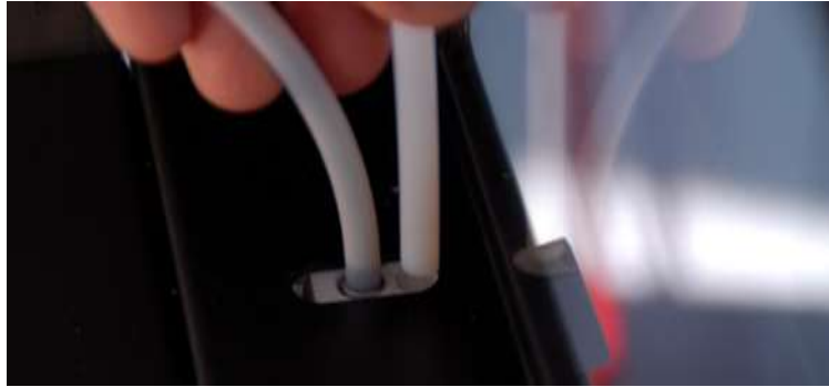
Figure 8.5.8 Fitting PTFE piping into motor assembly as shown
