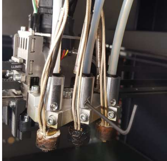
Figure 11.3.8 Using Set Screw to Secure Bowden Tube Adapter
