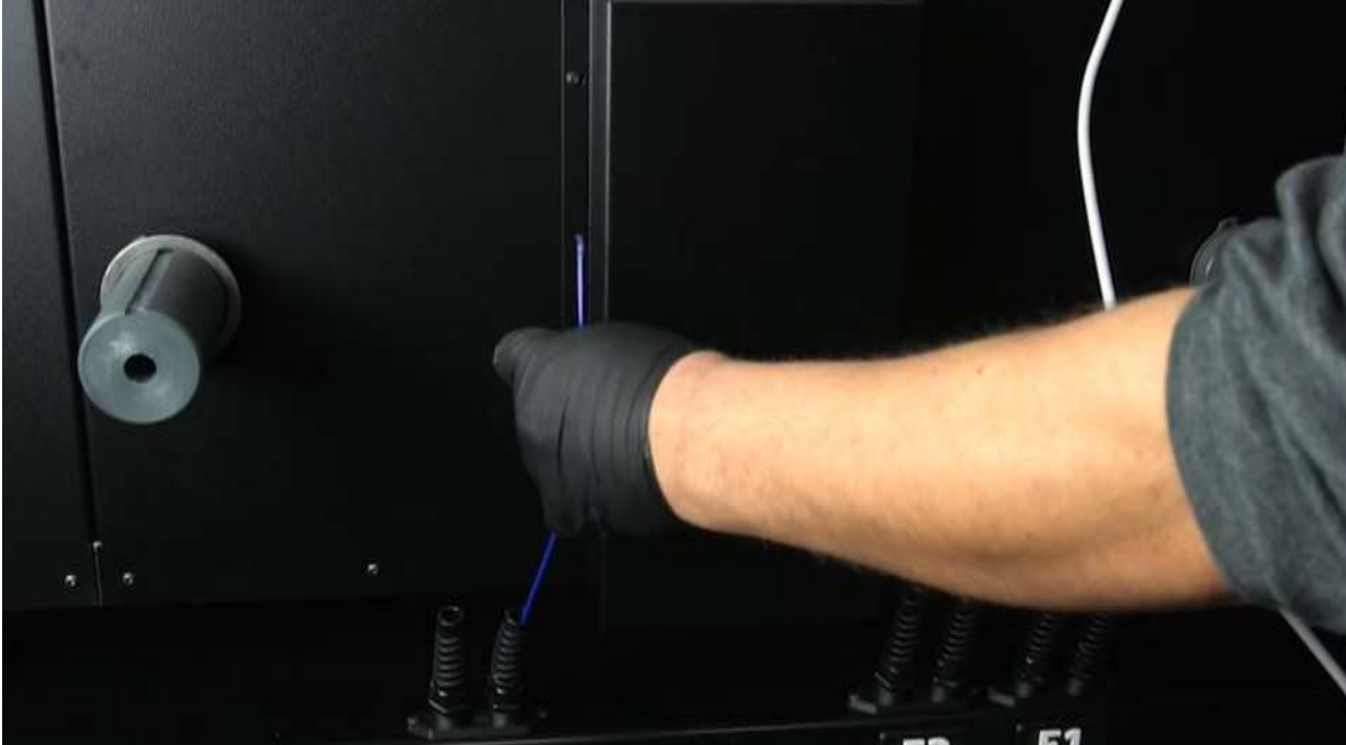
Figure 7.3.17 Pulling Filament from MMS up to Feeder
