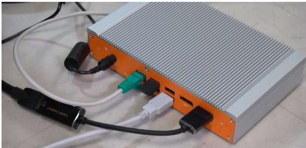
Figure 5.15.2 Print Server & Cable Connections – Typical for MMS Unit
