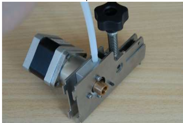
Figure 11.5.5 Fitting PTFE Pipe on Feeder
