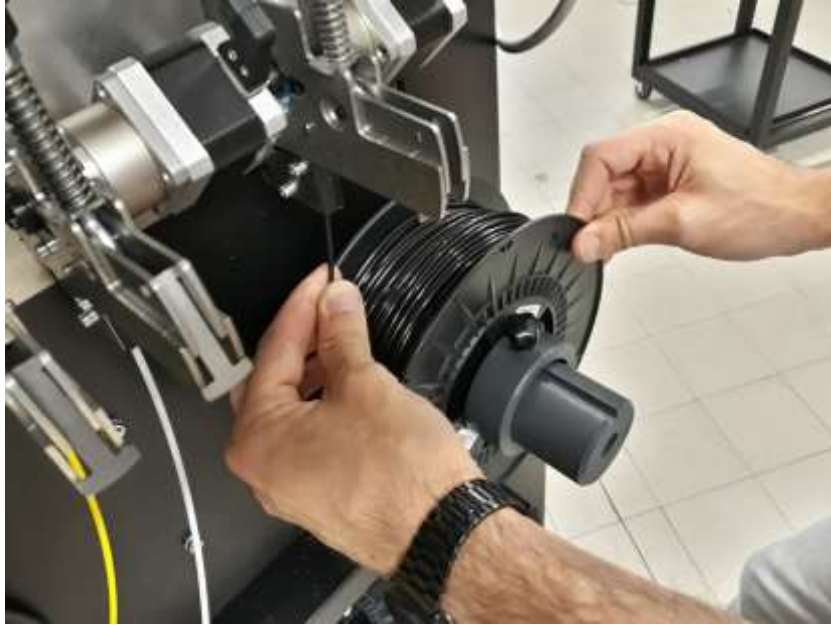
Figure 7.3.7 Pulling old filament out of feeder unit
