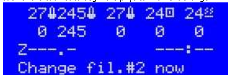
Figure 7.3.4 Heating/Purging Completed -Ready for Physical Filament Change
