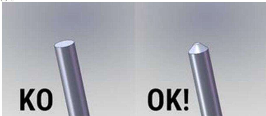
Figure 7.6.11 Illustration of correct and incorrect filament tip sharpening
