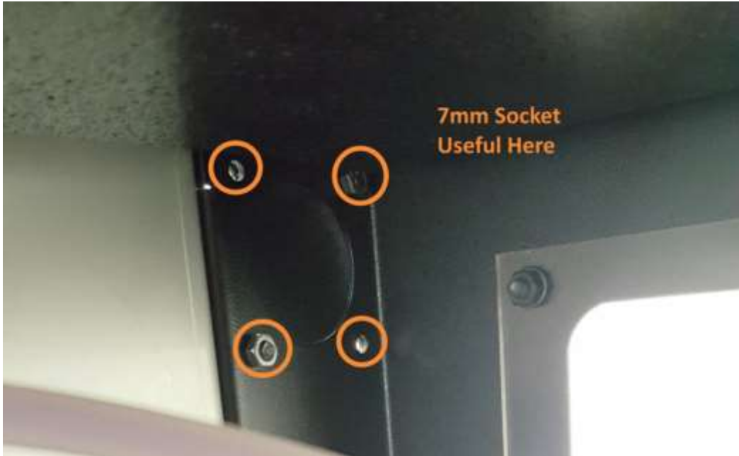
Figure 5.3.6 Blanking plate cover nuts in printer interior; hold with 7mm socket
