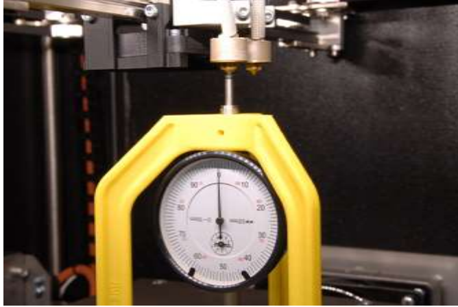
Figure 10.3.10 Dial Tip on Extruder #1 for Z Comparison
