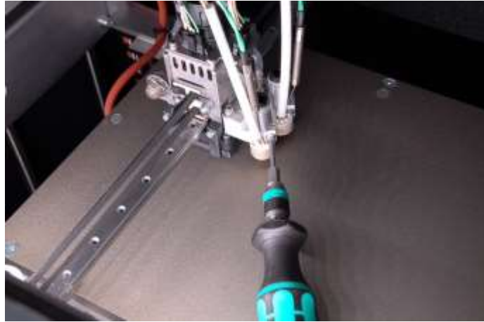
Figure 10.3.5 Locking Extruder #1 Set Screw to 1.3 Nm
