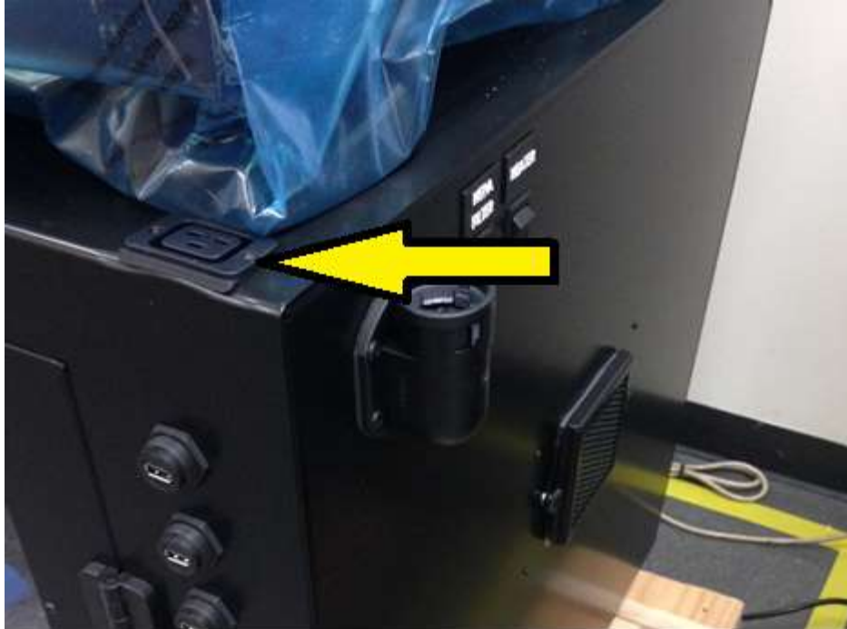
Figure 5.6.7 Printer power outlet on MMS Unit
