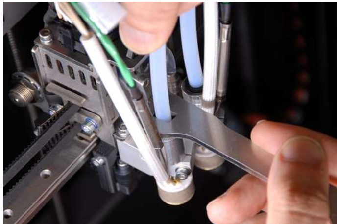
Figure 10.3.1 Remove PTFE Piping from Extruders
