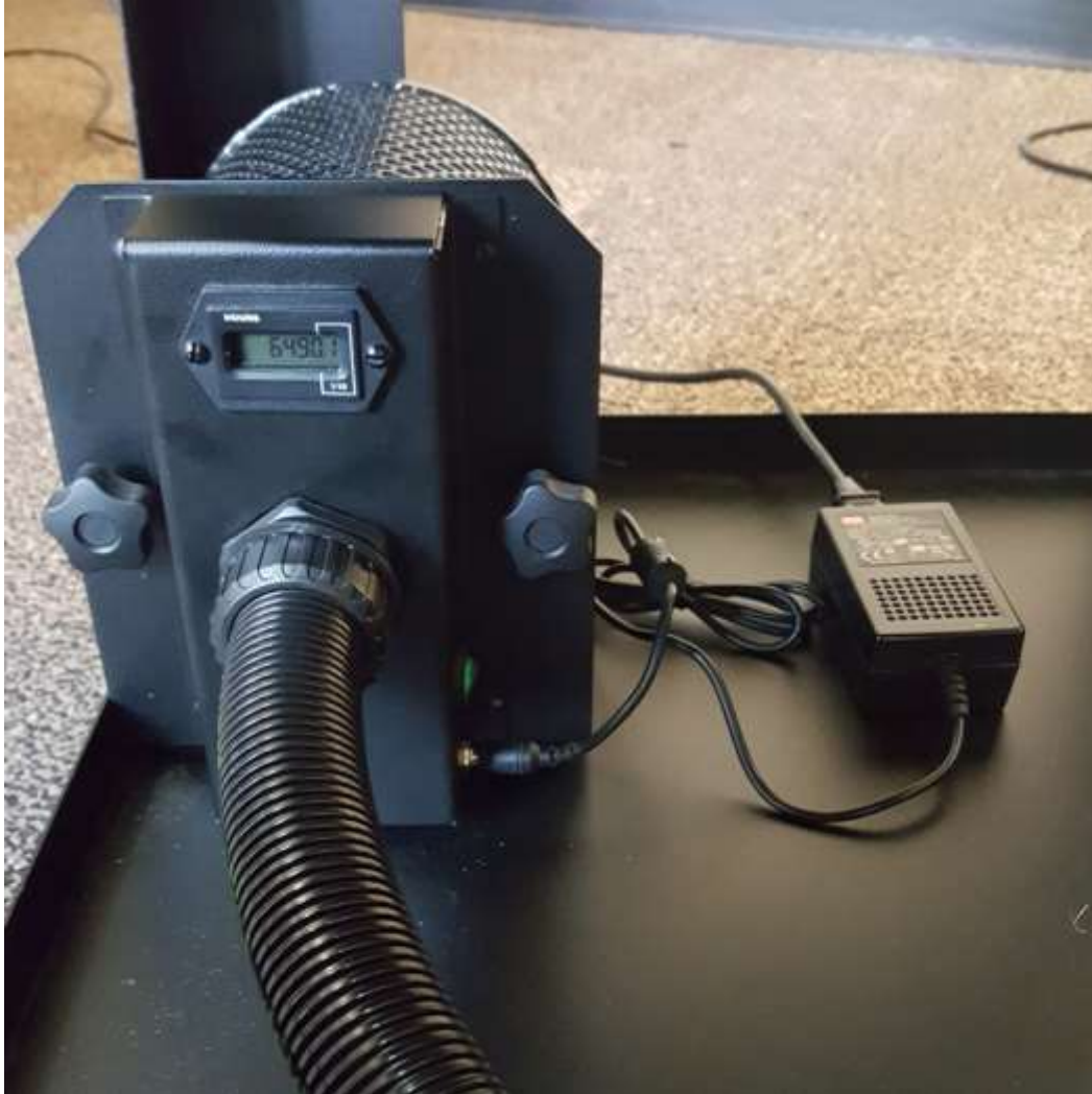
Figure 5.3.11 External HEPA Filter Unit Power Supply & Cord
