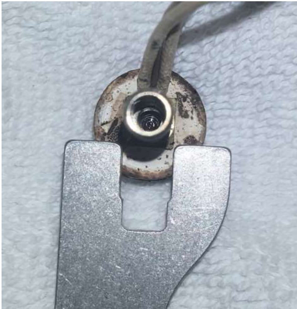
Figure 11.3.6 Custom Factory Supplied Tool for Gripping Square Surface
