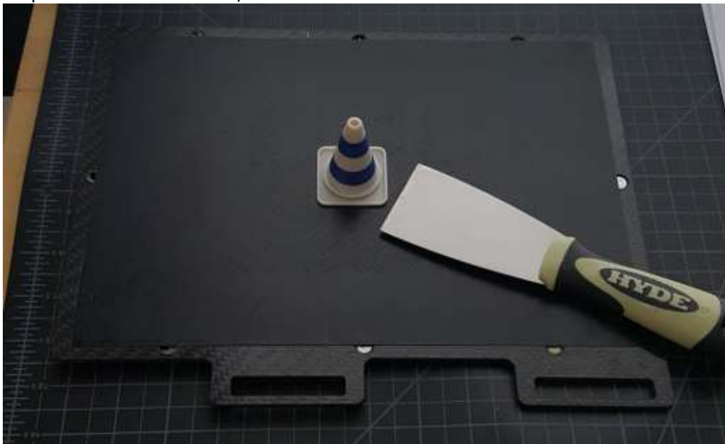
Figure 7.3 Printed Part (Cone) and supplied scraper tool
