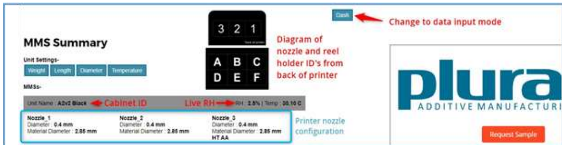
Figure 7.7.3 Locating the MMS Dash Button
