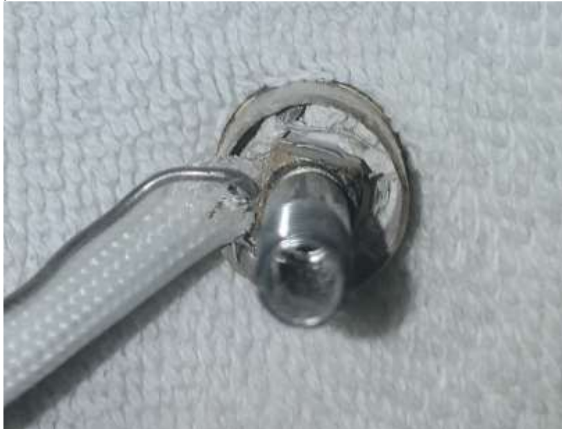
Figure 11.3.5 Damaged Ceramic Heater from Applied Force
