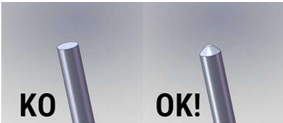
Figure 7.3.12 Illustration of correct and incorrect filament tip sharpening
