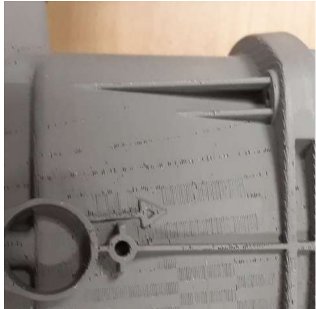
Figure 10.2.2 Print showing build and support material interference
