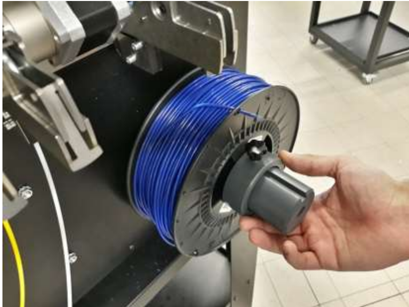
Figure 7.3.10 Install and secure a new filament spool
