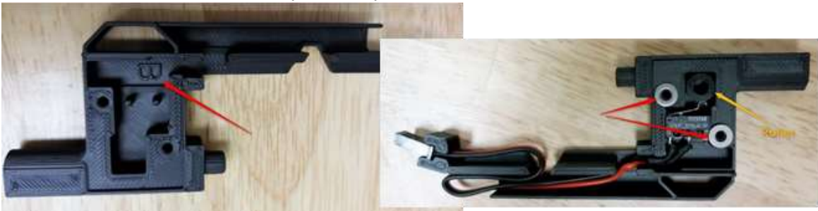
Figure 5.16.19 Spacer Installation (Only if No B/C on Sensor Body)
