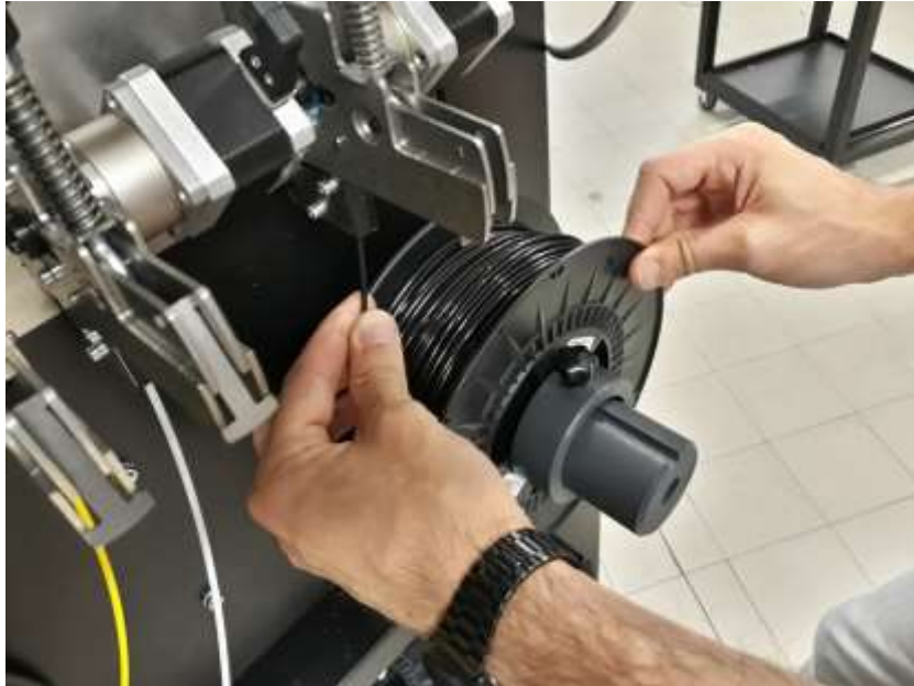
Figure 7.6.7 Pulling old filament out of feeder unit
