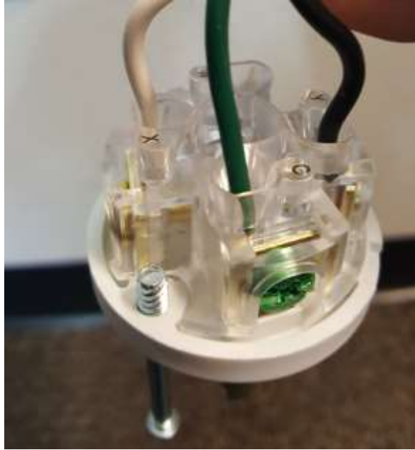
Figure 5.6.8 220 VAC Power Plug Wiring. Green = Ground. Black and White = 230 VAC single phase
