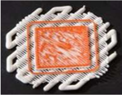
Figure 10.5.1 Extruder too High/Up: Redo Z Nozzle Leveling
