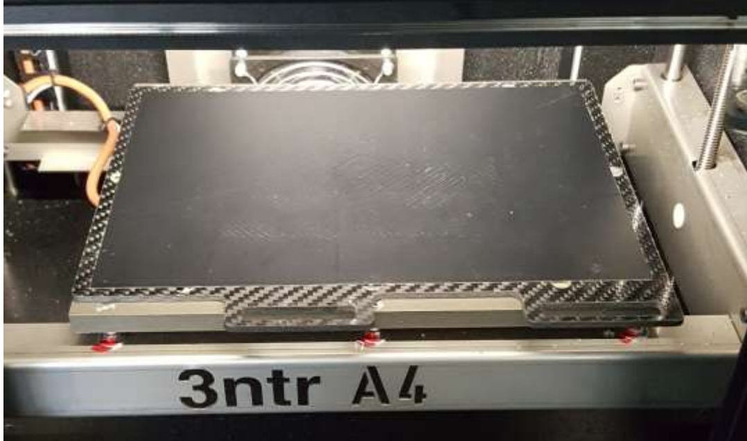
Figure 7.4 Printer surface plate re-installed in printer
