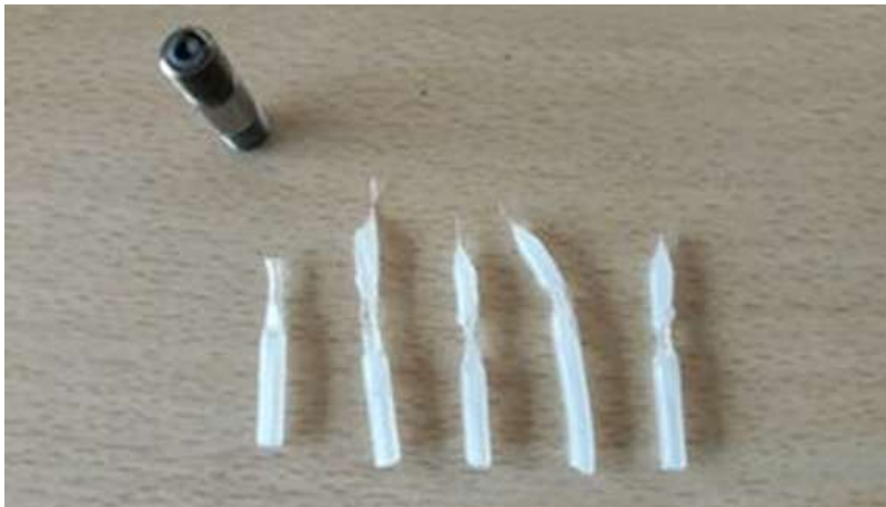
Figure 7.6.22 Bad Tips after Filament Cleaning: Requires Troubleshooting
