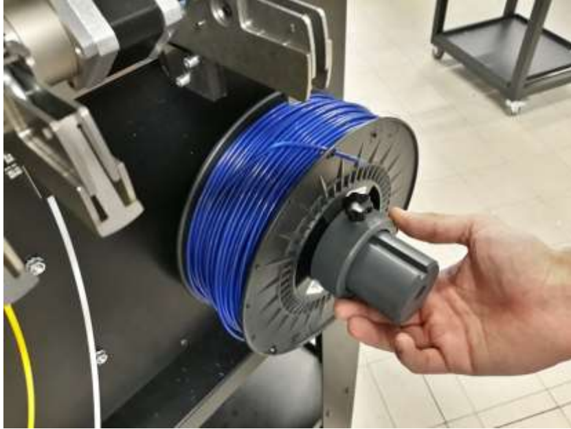
Figure 9.3.3 Install and secure a new filament spool
