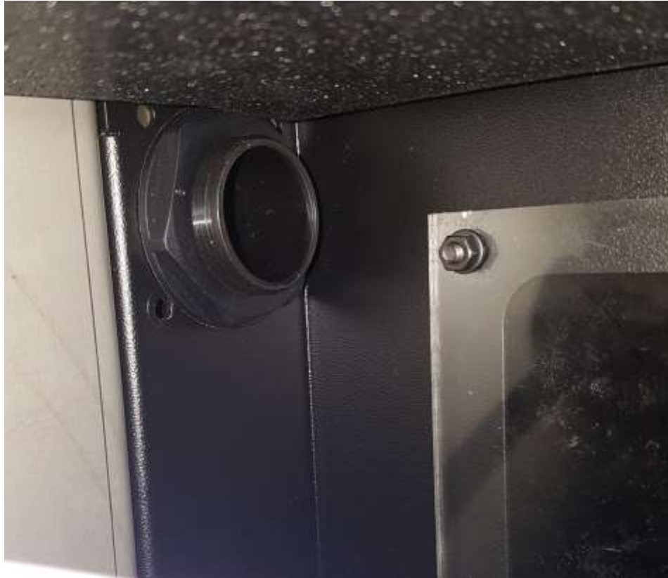
Figure 5.3.8 Interior View of Printer with Nut Retaining HEPA Filter Hose
