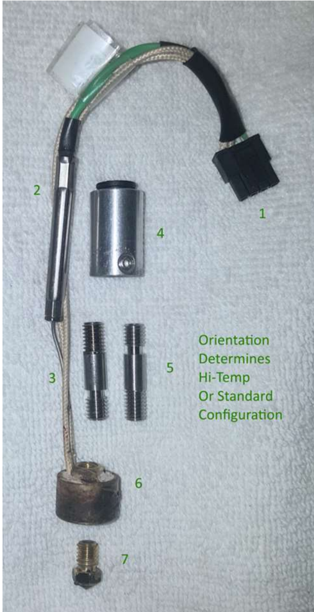
Figure 11.3.2 Extruder Component Identification Guide
