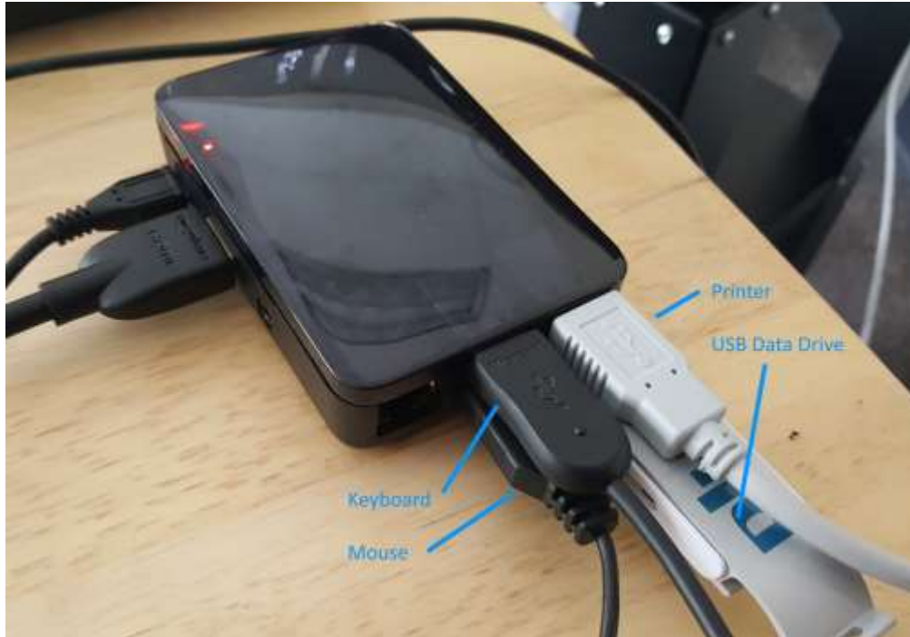
Figure 5.15.3 Cable Connections Locations for Print Server – No MMS
