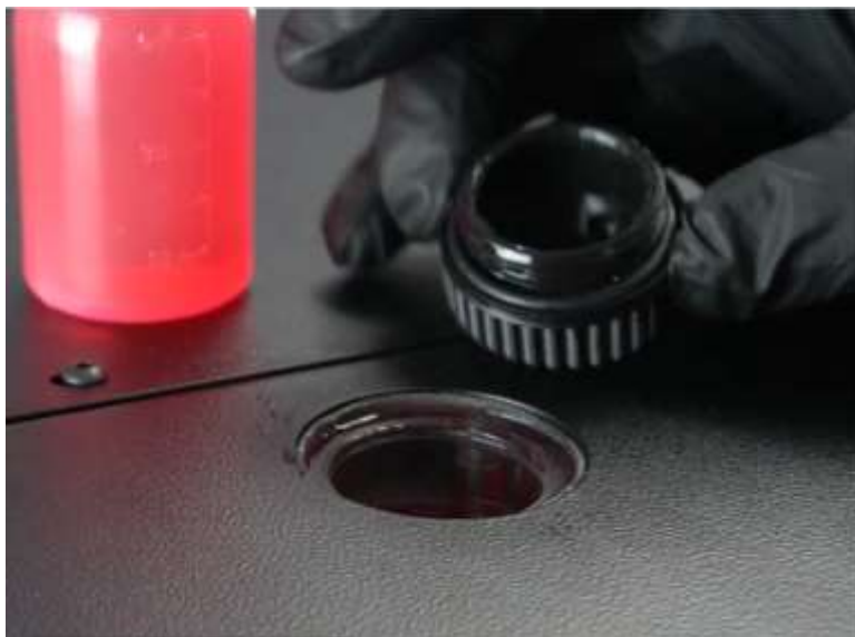
Figure 11.2.2 Proper Coolant Fill Level – \frac{1}{4} Inch Below Cap Thread
