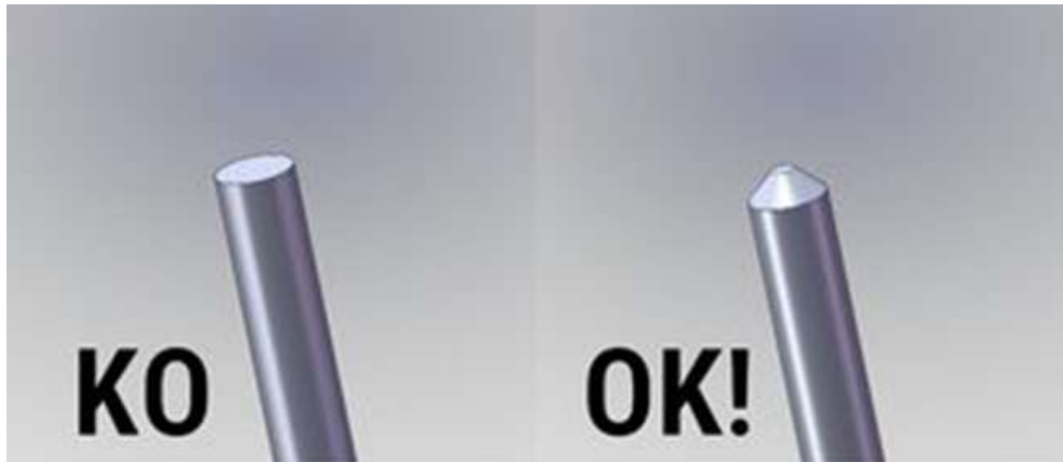
Figure 9.3.5 Illustration of correct and incorrect filament tip sharpening
