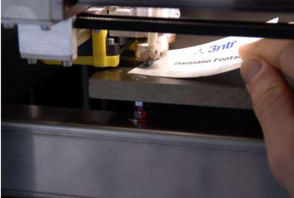
Figure 10.4.1 Using a Business Card to Assess Levelling
