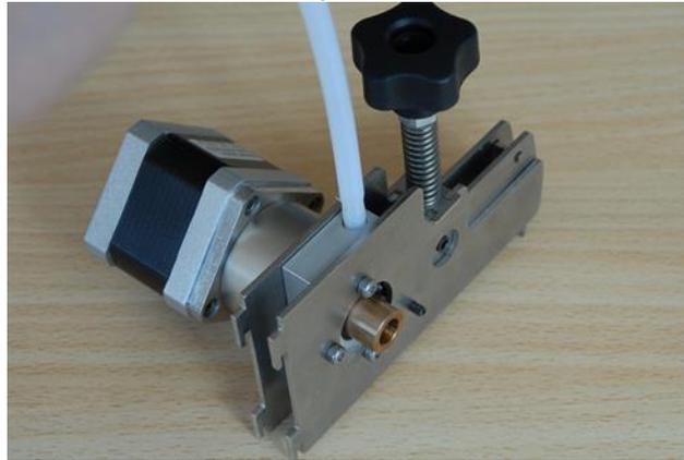
**Fitting PTFE Pipe on Feeder**
