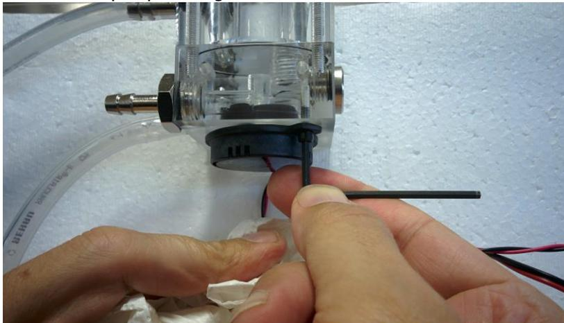
**Removing Pump/Reservoir Screws**
