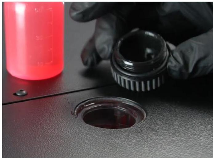
**Proper Coolant Fill Level –  $\frac{1}{4}$  Inch Below Cap Thread**
