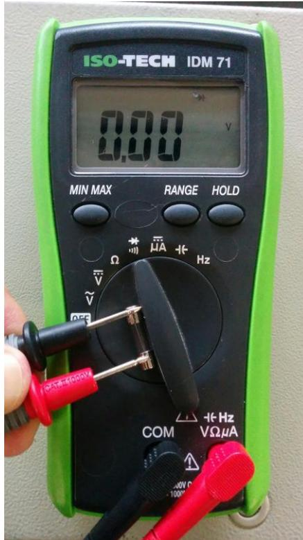
**Figure 6.23.4 Multimeter Indicating Fuse OK**
