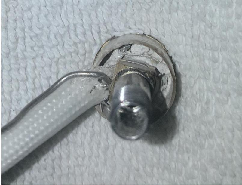
**Damaged Ceramic Heater from Applied Force**
