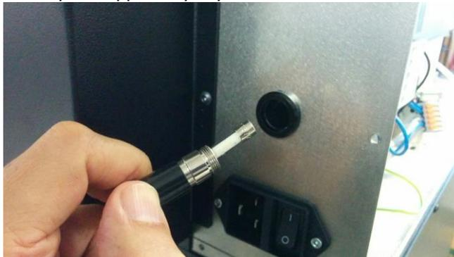
**Checking Fuse on Main Switch**
