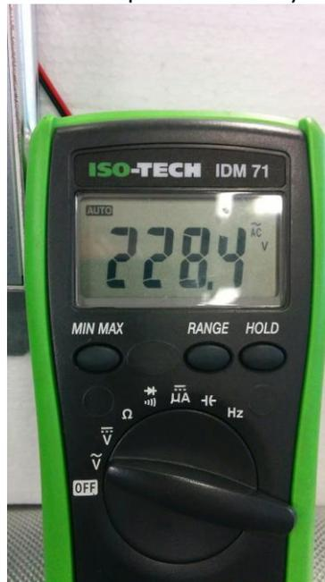
**Figure 6.24.2 Correct 228 VAC Entry – MM Set to AC**
