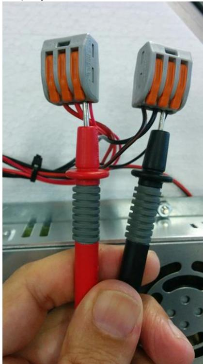
**Check PSU Output Voltage**
