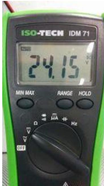
**Figure 6.24.4 Correct PSU DC Voltage Indicated on Multimeter**
