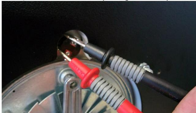
**Checking Safety Thermostat Current**
