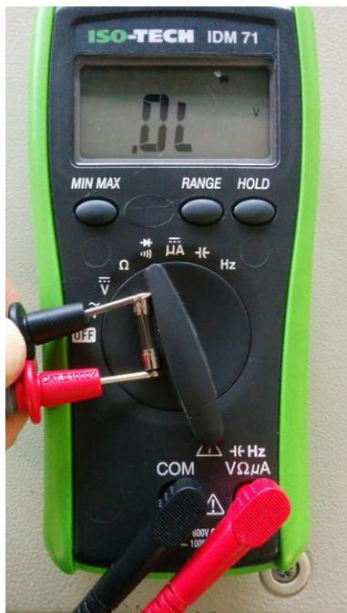
**Figure 6.23.3 Multimeter Indicating Blown Fuse**
