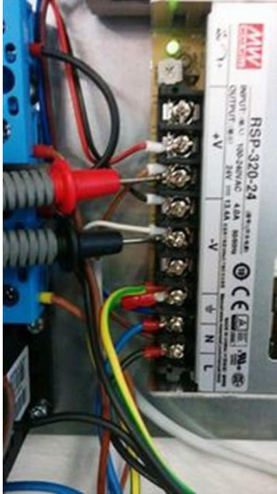
**Check Output Voltage on PSU**
