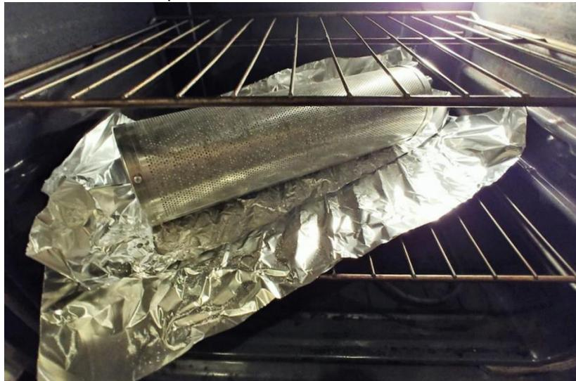
**Drying Desiccant Canister in Oven**
