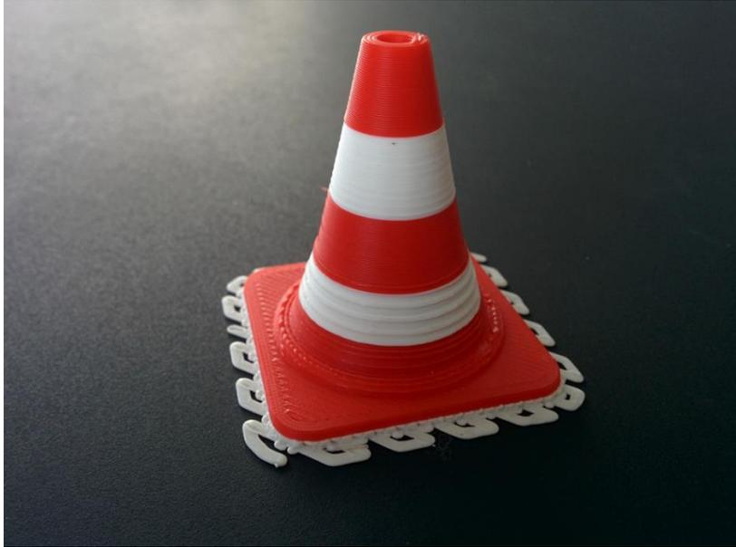
**Figure 6.16.1 Horizontal Banding on Lower Portion (Motherboard Fan Unplugged)**
