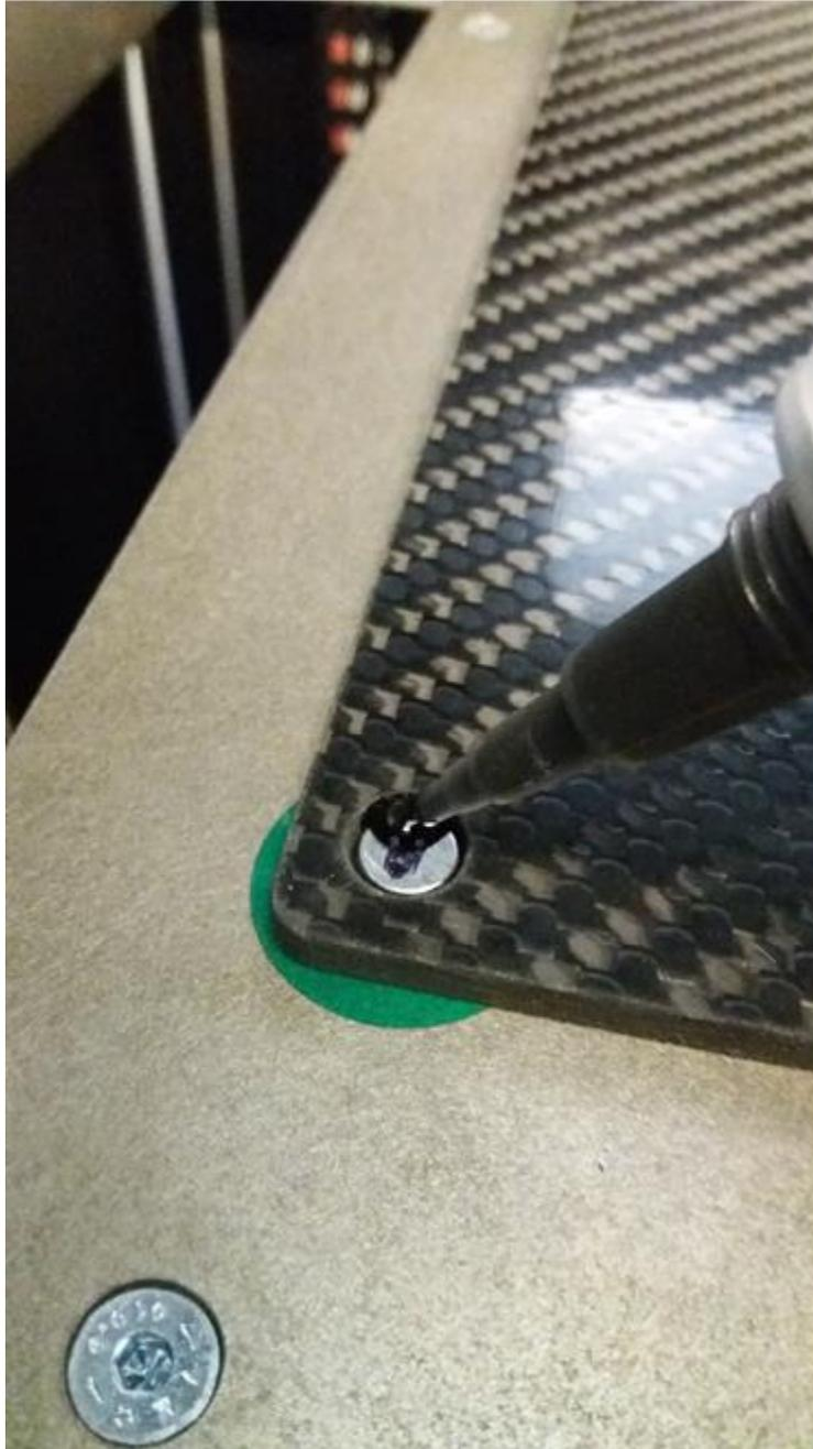
**Figure 6.21.7 Applying Glue to Magnet**
