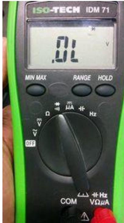
**Figure 6.23.1 Multimeter Set to Continuity Mode**
