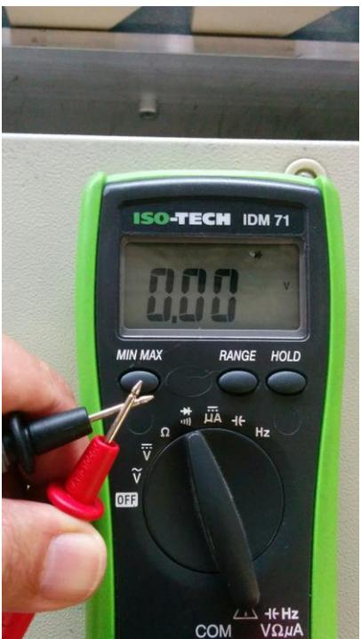
**Figure 6.23.2 Checking Multimeter Function – Touch Probes**
