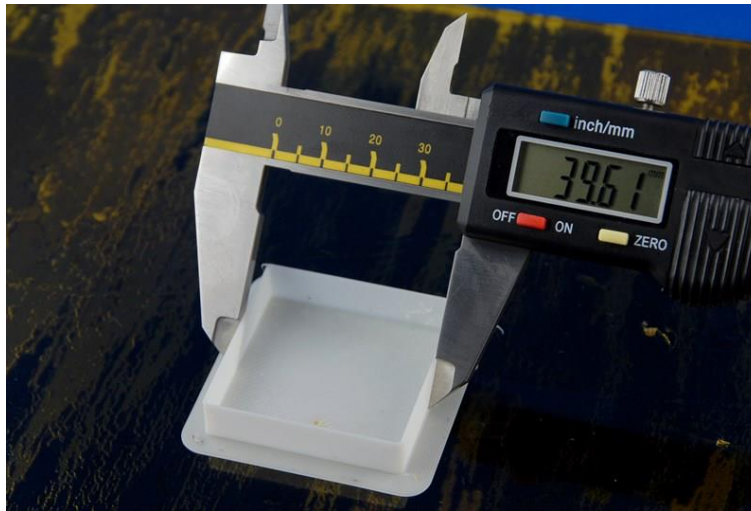
Fig. 64: Measure the printed part size along each axis
