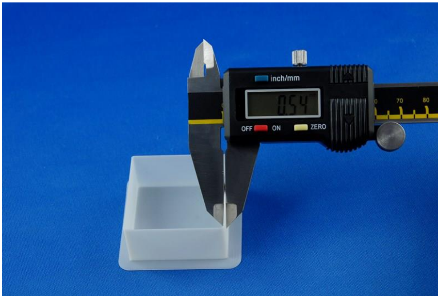
Fig. 63: Extrusion width measurement
