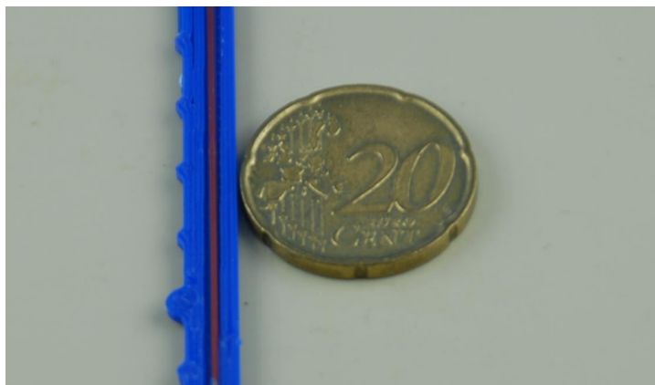
Fig. 73: X offset requires +0.1mm correction
