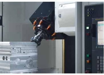
JapanTek 5X-410 features a tilting spindle head and CNCcontrolled rotary table that allows unrestricted five-sided machining of relatively large workpieces equal to the size of the 16" (406-mm) square table.
