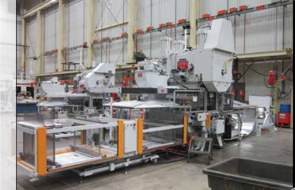
Burr Oak Tool makes equipment used in the production of HVAC systems. The progressive die press shown here is an example.
