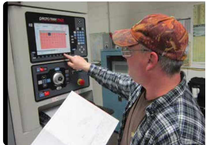
John Delarye, LPM lead man, programs a job using a conversational CNC. He attributes many of the company's gains in short-run production to control capabilities that streamline setup and change-over.
