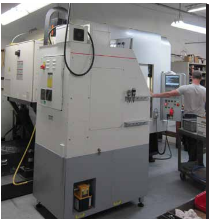
Chris Guidotti uses a pallet jack to maneuver the 20P CNC milling machine from Southwestern Industries into position near one of the shop's Brother VMCs. The shop has additional electrical drops near all primary lathes and mills to enable the portable machine to be located wherever a mini cell is needed.
