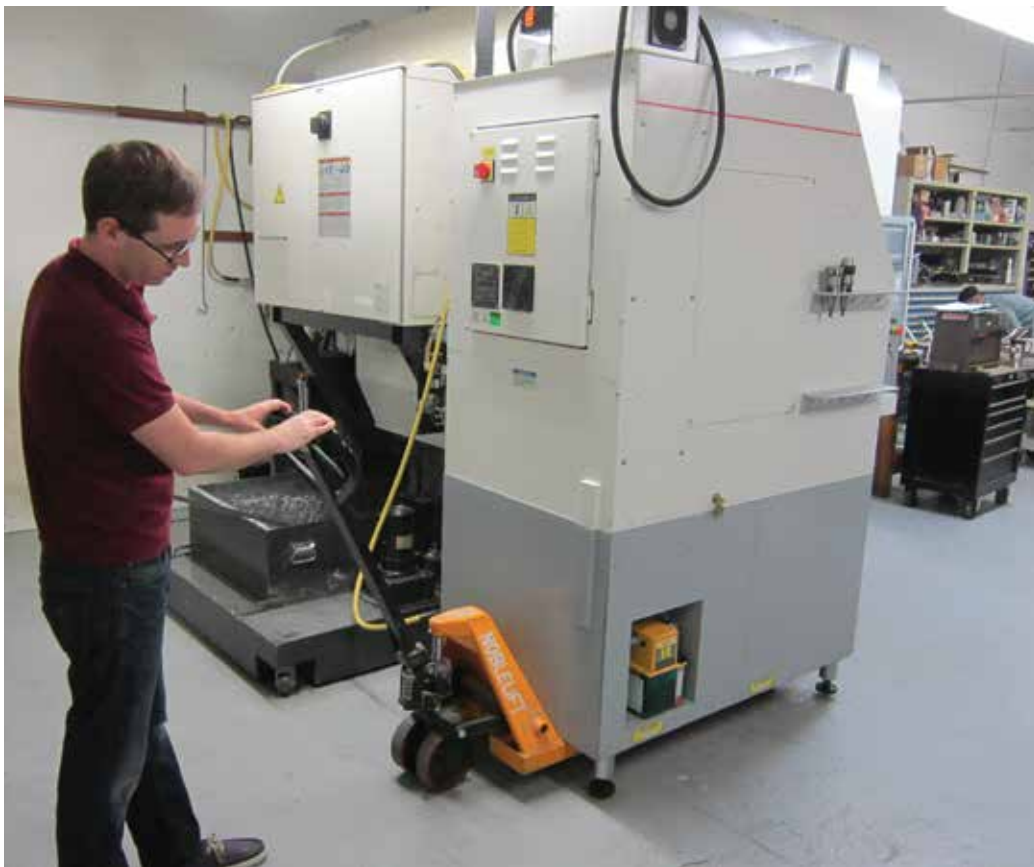
Chris Guidotti uses a pallet jack to maneuver the 20P CNC milling machine from Southwestern Industries into position near one of the shop's Brother VMCs. The shop has additional electrical drops near all primary lathes and mills to enable the portable machine to be located wherever a mini cell is needed.
