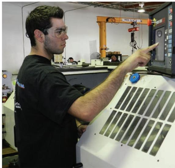
**Claudio Gamez Jr., Machine Operator, working with the ProtoTRAK control on a Southwestern Industries 2460SX lathe.**
