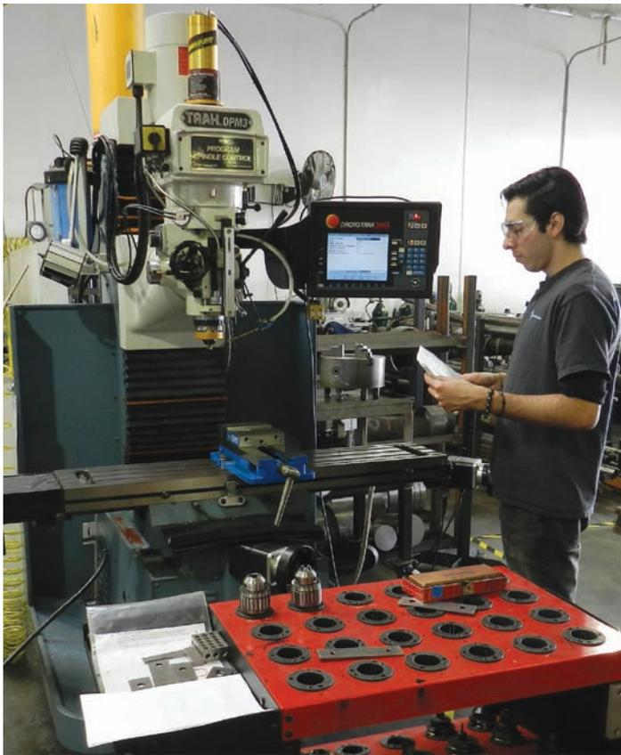
**Hector Gamez, Machine Operator, working at a TRAK model DPMSX3P bed mill with ProtoTRAK SMX CNC control.**
