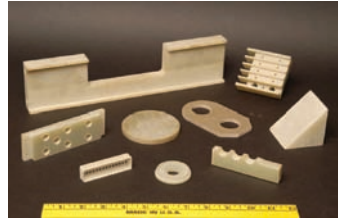
UHMW parts machined at Moore-Addison.
