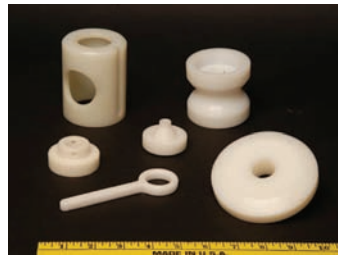
Delrin parts machined at Moore-Addison.
