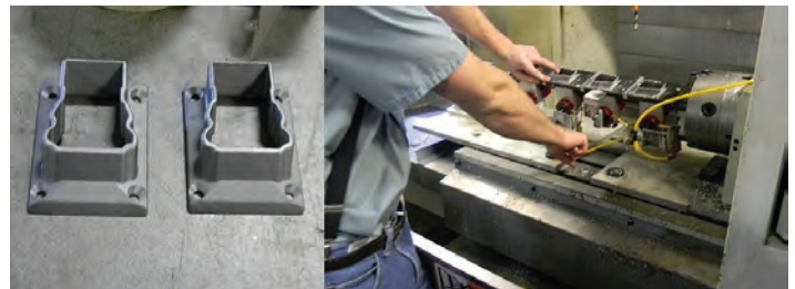
Stair brackets machined using the LPM's 4th axis capabilities.
