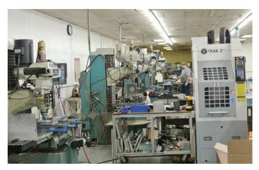
TRAK 2<sup>OP</sup> placed next to CNC mills for simultaneous machining of two different parts.
